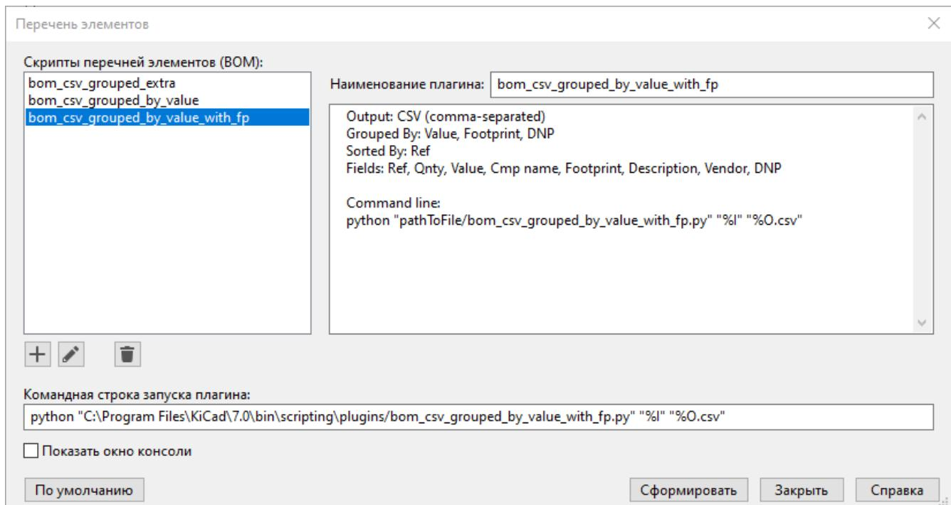
KiCad has a GUI for BOM export. You can configure which symbol metadata will be exported, and how the symbols are grouped, in the **Edit** tab, and configure the output format in the **Export** tab.
