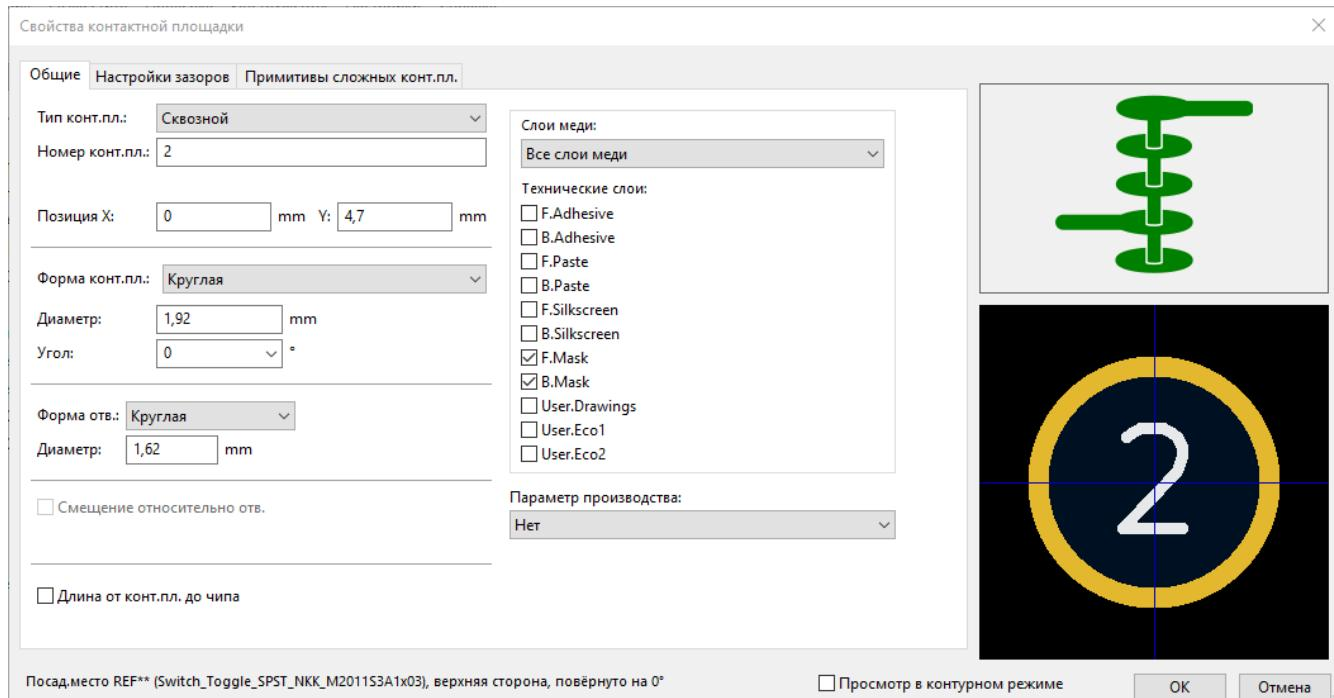
Now use the **Add a pad** tool again to place the other pad at (0, 9.4 mm). Notice that the pad number is automatically incremented and the properties including pad size and hole size are copied from the previous pad.
