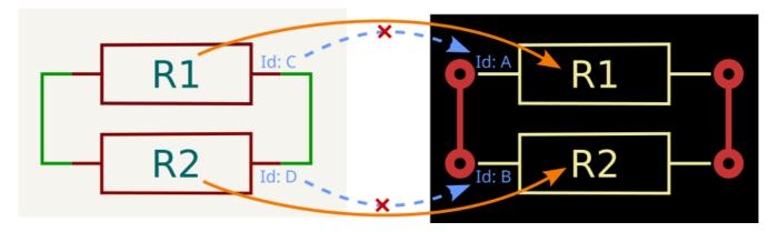
Re-linking the footprints by reference designator causes KiCad to re-create the links, using the matching reference designators as a guide.
