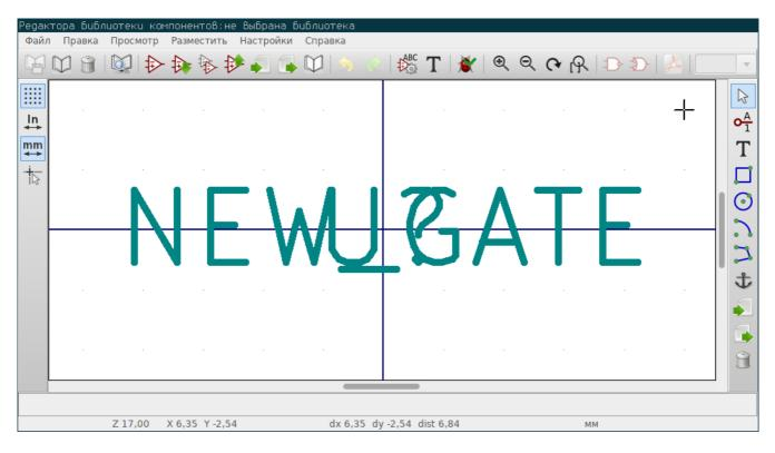
The blue cross in the center is the symbol anchor, which specifies the symbol origin i.e. the coordinates (0, 0). The anchor can be repositioned by selecting the 4000 button and clicking on the new desired anchor position.
