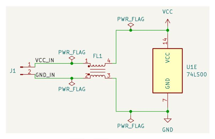
This would be the case also if the VCC\_IN and GND\_IN nets were connected to a symbol with Output Power pins. In fact, in this schematic, the PWR\_FLAG symbols are on VCC\_IN and GND\_IN are not required, as there are no Input Power pins on those nets.
