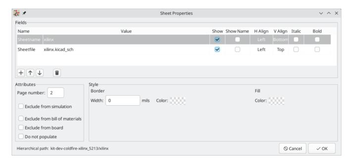
The **sheet name** must be unique, as it is used in the full net name for any nets in the subsheet. For example, a net with the local label net1 in the sheet sheet1 would have a full net name of /sheet1/net1. The sheet name is also used to refer to the sheet in various places in the GUI, including the title block and the hierarchy navigator. The sheet name can also be changed in the hierarchy navigator.
