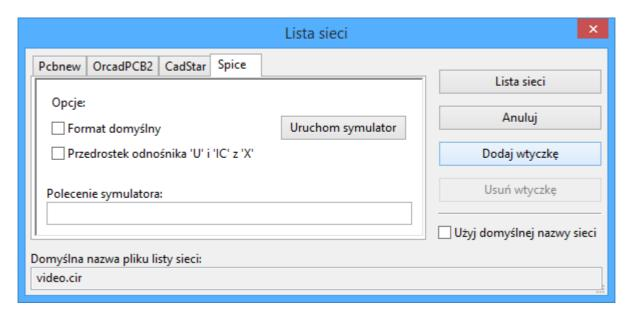
New generators require a name and a command. The name is shown in the tab label, and the command is run whenever the **Export Netlist** button is clicked.
