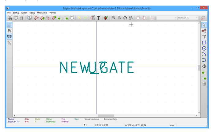
The blue cross in the center is the symbol anchor, which specifies the symbol origin i.e. the coordinates (0, 0). The anchor can be repositioned by selecting the \* button and clicking on the new desired anchor position.
