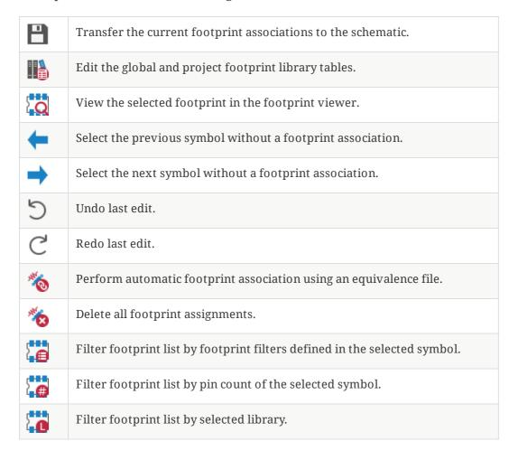
The following table lists the keyboard commands for the Footprint Assignment Tool:
