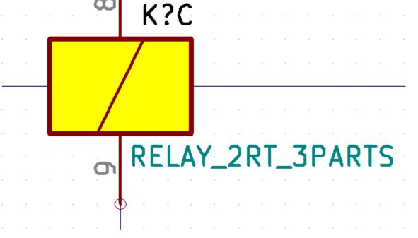
Unit A does not have the same symbol and pin layout as Units B and C, so the units are not interchangeable.
