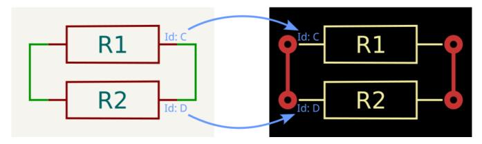
Because the links have been re-established, the next forward annotation should use the normal identifier-based linking (i.e. the checkbox should be unchecked).
