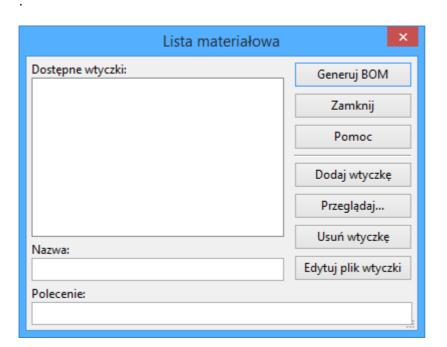
Several BOM generator scripts are included with KiCad, and users can also create their own. BOM generator scripts generally use Python or XSLT, but other tools can be used as long as you can specify a command line for KiCad to execute when running the generator.
