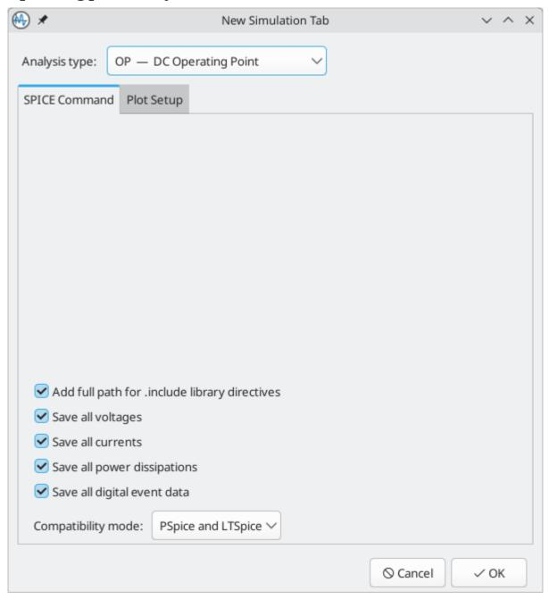
Calculates the DC operating point of the circuit. This analysis has no options.
