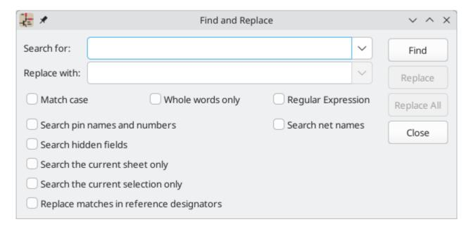
The Find and Replace tool has the same options as the Find tool, with one addition:
