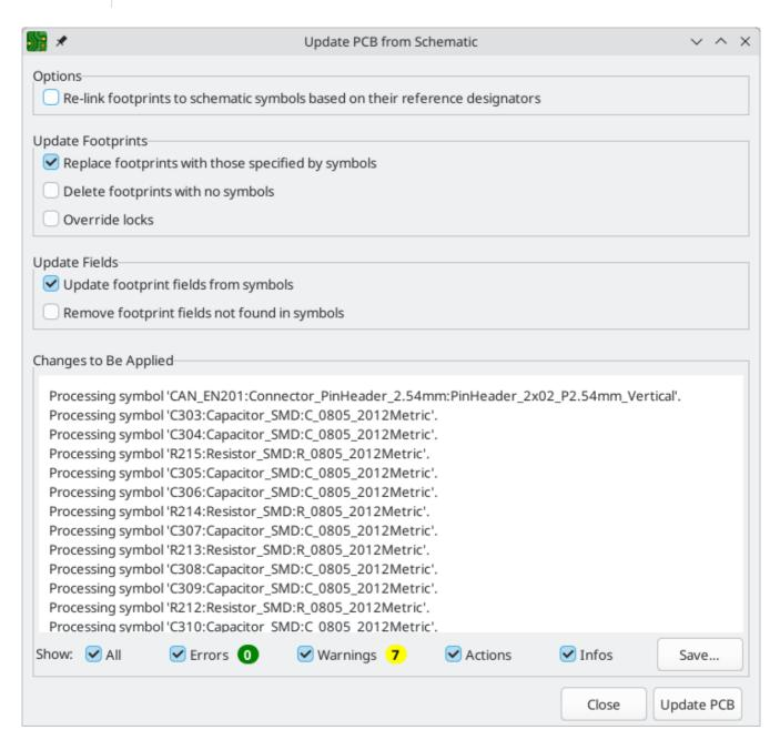
The tool adds the footprint for each symbol to the board and transfers updated schematic information to the board. In particular, the board's net connections are updated to match the schematic. Symbols with the Exclude from board attribute are not transferred to the PCB.
