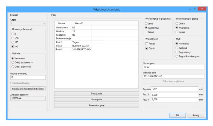
The Symbol Properties window displays all the fields of a symbol in a table. New fields can be added, and existing fields can be deleted, edited, reordered, moved, or resized. Fields can be arbitrarily named, but names beginning with ki\_, e.g. ki\_description, are reserved by KiCad and should not be used for user fields. All symbol fields will be added to the symbol's corresponding footprint when the PCB is updated from the schematic.
