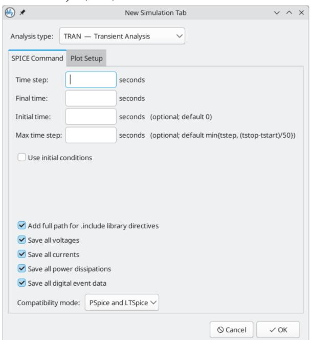
Calculates the time-varying behavior of the circuit.
