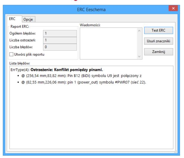
Any warnings or errors are reported in the **Violations** tab, and markers for each violation are placed in the schematic so that they point to the relevant part of the schematic. Warnings are indicated by yellow arrows, and errors have red arrows. Excluded violations are shown as green arrows. A list of the ignored tests are
