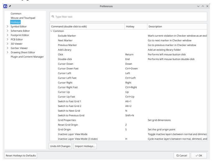
You can use this dialog to customize the hotkeys used to control KiCad. The hotkeys in the *Common* section are shared between every KiCad program. Hotkeys for each specific KiCad program are shown when that program is running. You can assign the same hotkey to a different action in different KiCad programs (for example, the schematic editor and the board editor), but you cannot assign a hotkey to more than one action in the same program.
