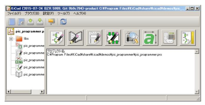
The KiCad project manager window is composed of a tree view on the left showing the files associated with the open project, and a launcher on the right containing shortcuts to the various editors and tools.
