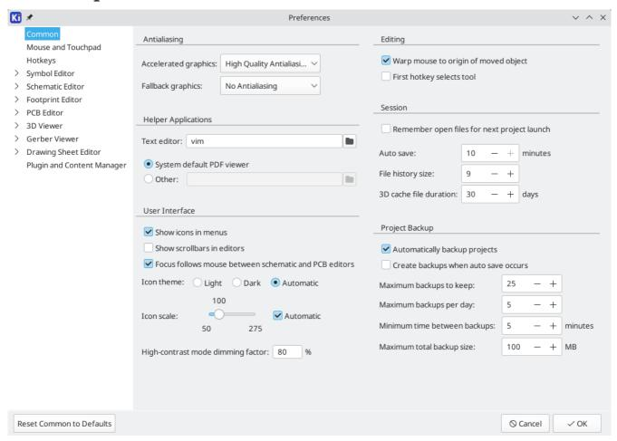
Accelerated graphics antialising: KiCad can use different methods to prevent aliasing (jagged lines) when rendering using a graphics card. Different methods may look better on different hardware, so you may want to experiment to find the one that looks best to you.
