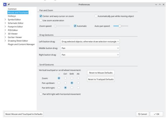
**Center and warp cursor on zoom:** When enabled, zooming using the hotkeys or mouse wheel will cause the view to be centered on the cursor location.
