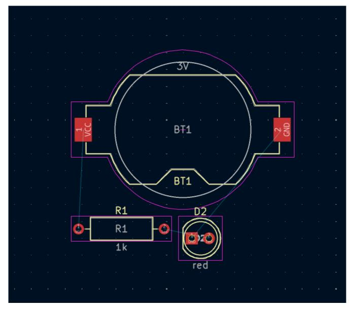
In KiCad, updating the PCB with changes in the schematic is a manual process: the designer decides when it is appropriate to update the PCB with modifications in the schematic. Each time the schematic is edited, the designer must use the **Update PCB from Schematic** tool to keep the schematic and layout in sync.
