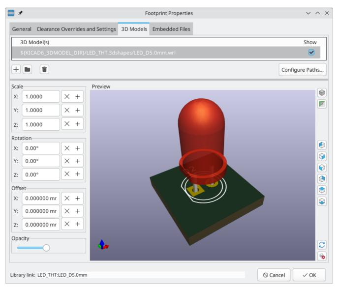
Both STEP (.step) and VRML (.wrl) 3D model formats are supported. STEP files are useful where dimensional accuracy is needed, while VRML files can be used for more visually attractive renders. Many footprints in KiCad's library have associated 3D models; these models are provided in both VRML and STEP formats. Only one of the two models needs to be listed in the footprint (typically the VRML filename is
