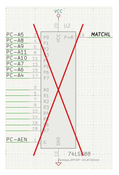
To edit the symbols's form, i.e. its pins and graphics, you need to use the symbol editor. There are two buttons for opening a symbol in the editor, depending on whether you want to edit a single copy of a symbol in the schematic or a symbol's source copy in the library.
