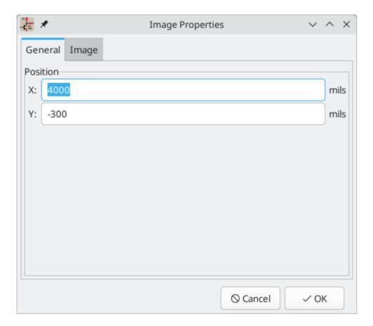
You can also reposition or scale the image in its properties dialog (**E**). You can set the image's exact **Position X** and **Y** in the **General** tab, and set an exact **Scale** factor in the **Image** tab. You can also **Convert to Greyscale** if you wish. Position and scale in this dialog are relative to the center of the image, not its interactive reference point.
