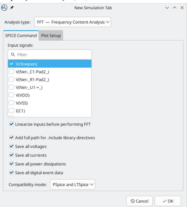
Calculates an FFT based on an existing analysis tab. Any of the signals from an existing analysis can be used as inputs to the FFT. The signals are windowed using a Hanning window.
