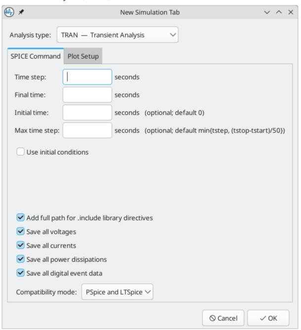
Calculates the time-varying behavior of the circuit.
