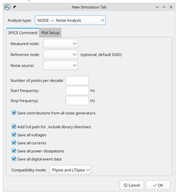
Calculates the noise generated by the devices in the circuit, both as output noise and input-referred noise. The noise spectrum (V/ $\sqrt{Hz}$  or A/ $\sqrt{Hz}$ ) of the circuit can be plotted, and the total noise over the specified frequency range is reported. Optionally, the noise contributions of each device are reported individually.
