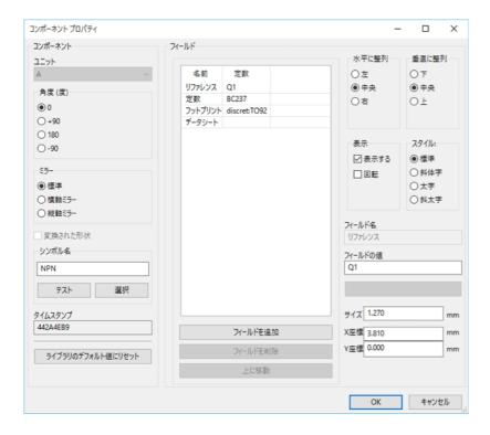
The Symbol Properties window displays all the fields of a symbol in a table. New fields can be added, and existing fields can be deleted, edited, reordered, moved, or resized. Fields can be arbitrarily named, but names beginning with ki\_, e.g. ki\_description, are reserved by KiCad and should not be used for user fields. All symbol fields will be added to the symbol's corresponding footprint when the PCB is updated from the schematic.
