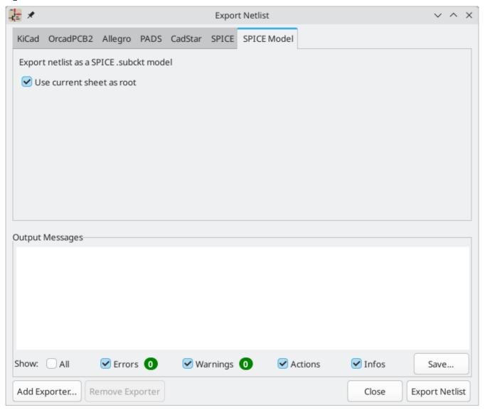
KiCad can also export a netlist of the schematic as a Spice subcircuit model, which can be included in a separate Spice simulation. Any hierarchical labels in the schematic are used as pins for the subcircuit model. Each pin in the model is annotated with a comment describing the pin's electrical direction:
