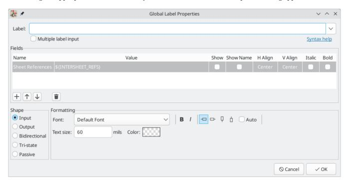
The **Label** field sets the label's text, which determines the net that the label assigns to its attached wire. You can choose a label name from a list of nets that are already in the schematic by clicking the dropdown menu next to the label name field.
