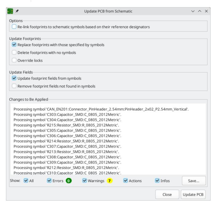
The tool adds the footprint for each symbol to the board and transfers updated schematic information to the board. In particular, the board's net connections are updated to match the schematic. Symbols with the
