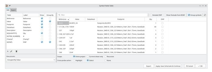
Fields with the **Show** box checked will be included as columns in the BOM, and fields with the **Group By** box checked are used to group components together. Components are grouped into the same line if all of their **Group By** fields are identical and the **Group symbols** box is checked. You can set an arbitrary column name for each field and reorder columns by dragging their headers.
