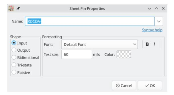
The sheet pin's **name** can be edited in the textbox or by selecting from the dropdown list of hierarchical labels in the subsheet. A sheet pin's name has to match the corresponding hierarchical label in the subsheet, so if you change a pin name you must change the label name as well.
