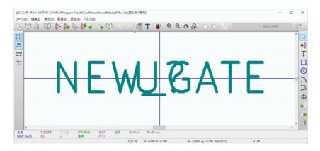
The blue cross in the center is the symbol anchor, which specifies the symbol origin i.e. the coordinates (0, 0). The anchor can be repositioned by selecting the hour and clicking on the new desired anchor position.
