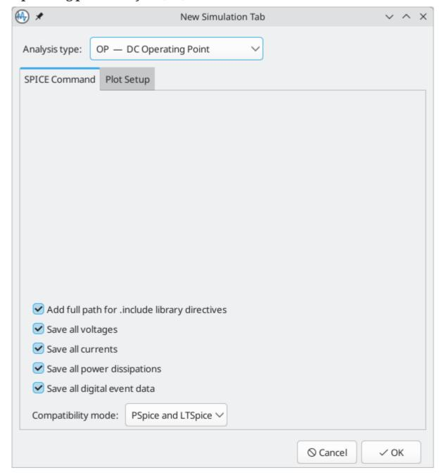
Calculates the DC operating point of the circuit. This analysis has no options.
