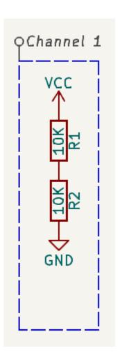
Components can have more than one class, and symbols take on a class if any of their sub-units have that class. If multiple Component Class fields are added to a directive label, or multiple directive labels with Component Class fields are applied to a rule area, the symbols in the rule area will take on all of the specified component classes.
