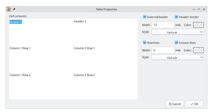
This dialog lets you edit the properties of the entire table, including the text in each cell and the separators between cells. To change the formatting of text in a cell, edit the properties of individual cells, instead of the properties for the entire table.
