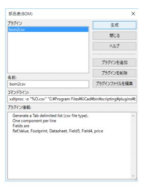
Additional scripts can be added to the list of BOM generator scripts by clicking the + button. Scripts can be removed by clicking the  $\uparrow$  button. The  $\nearrow$  button opens the selected script in a text editor.
