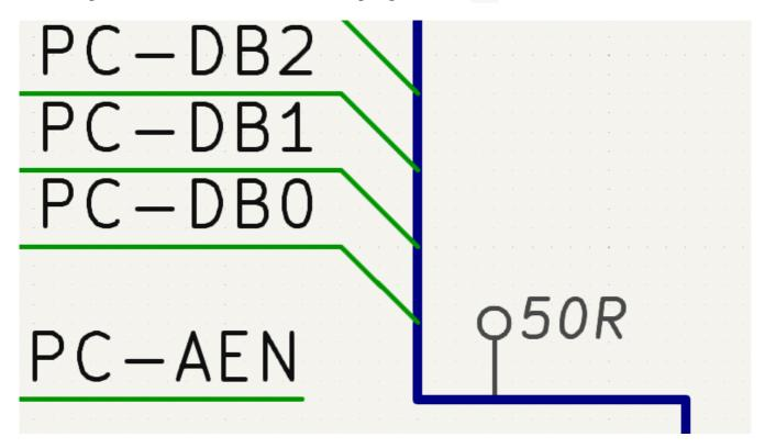
Directive labels are added with the QA button in the right toolbar. They behave like labels, except that they cannot be used to name a net. The attached net is assigned a net class according to the value of the directive's
