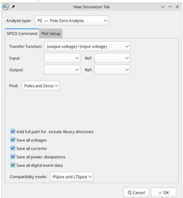
Calculates the poles and zeroes of the small-signal (AC) transfer function of the circuit.
