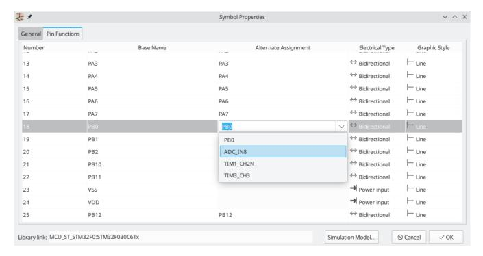
Pins that have alternate functions available are displayed with a small graphical indicator next to the pin name, as shown in the screenshot below. To globally show or hide these indicators, use  $\mathbf{View} \rightarrow \mathbf{Show}$  **Pin** Alternate Icons.
