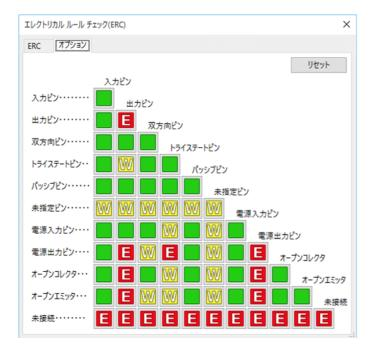
Rules can be changed by clicking on the desired square of the matrix, causing it to cycle through the choices: allowed, warning, error.
