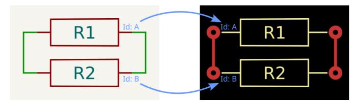
If symbol reference designators are changed in the schematic (e.g. by re-annotation), running the **Update PCB from Schematic** process will update the reference designators on the PCB.
