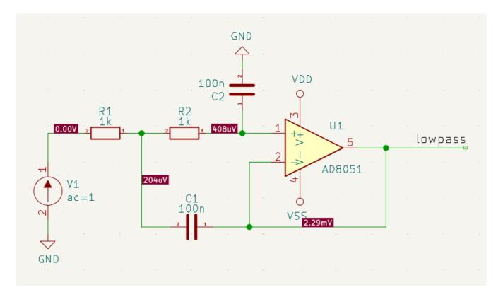
You can also display operating point results using text variables. Using text variables requires more work to set up but provides more control over how the data is displayed. For example, you can use text variables to display only certain voltages or currents, or to control the display formatting of particular values. You can also use text variables to display power dissipation measurements.
