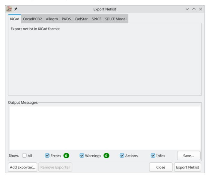
KiCad supports exporting netlists in several formats: KiCad, OrcadPCB2, Allegro, PADS, CADSTAR, Spice, and Spice Model. Each format can be selected by selecting the corresponding tab at the top of the window. Some netlist formats have additional options.
