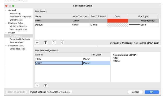
The **Net Classes** panel allows you to manage net classes for the project and assign nets to net classes with patterns. Managing net classes in this panel is equivalent to managing them in the Board Setup dialog. Nets can also be assigned to net classes in the schematic using graphical assignments with net class directives or net labels.
