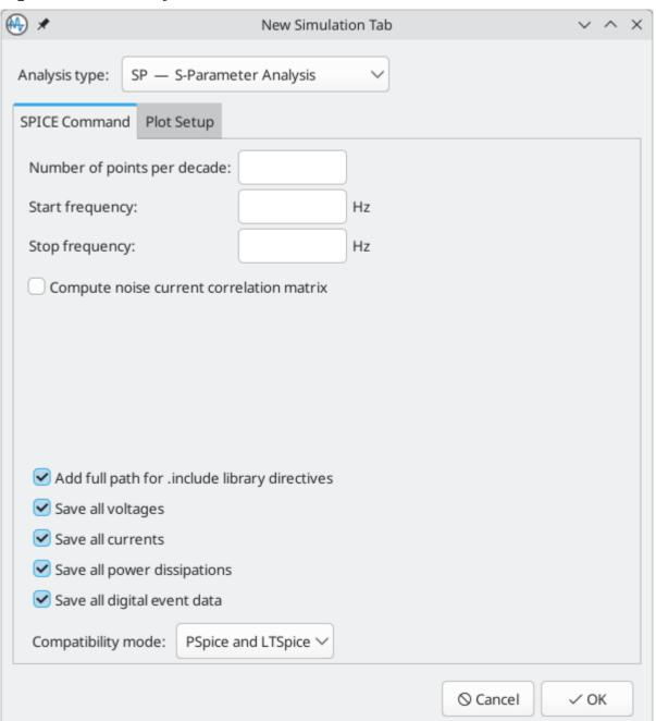
Calculates the scattering parameters, admittance matrix, and impedance matrix for the circuit. Optionally calculates the noise current correlation matrix. Note that this analysis requires at least two voltage sources configured as RF ports as described in the ngspice manual.
