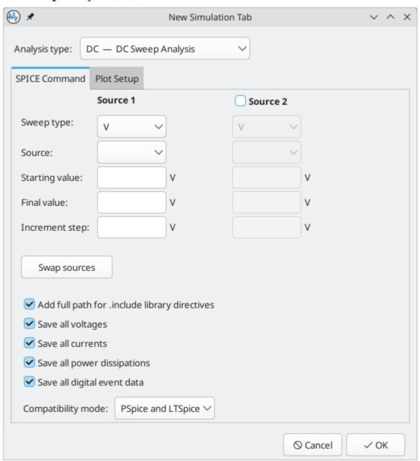
Calculates the DC behavior of the circuit while sweeping one or two parameters. The following parameters can be swept:
