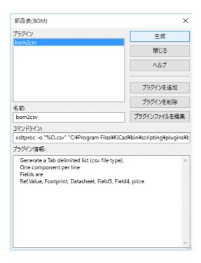
Several BOM generator scripts are included with KiCad, and users can also create their own. BOM generator scripts generally use Python or XSLT, but other tools can be used as long as you can specify a command line for KiCad to execute when running the generator.
