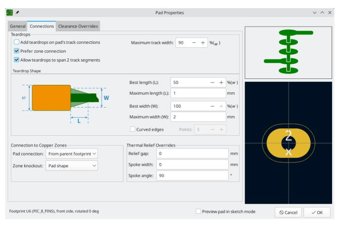
Teardrops in KiCad are small zones, meaning that when they refill they avoid shorting to copper objects on other nets. They are initally filled when they are added, but they are unfilled and refilled with other zones on the board: when using the Unfill All Zones and Refill All Zones commands, running DRC, generating fabrication outputs, etc. Teardrops can be shown in filled or outline mode using the zone display controls in the left toolbar.
