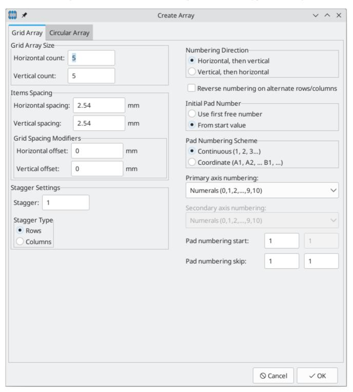
For grid arrays, you can select a numbering direction, either **horizontal**, **then vertical** or **vertical**, **then horizontal**. If **reverse numbering on alternate rows/columns** is selected, the direction of increasing pad numbers will alternate from one row/column to the next.
