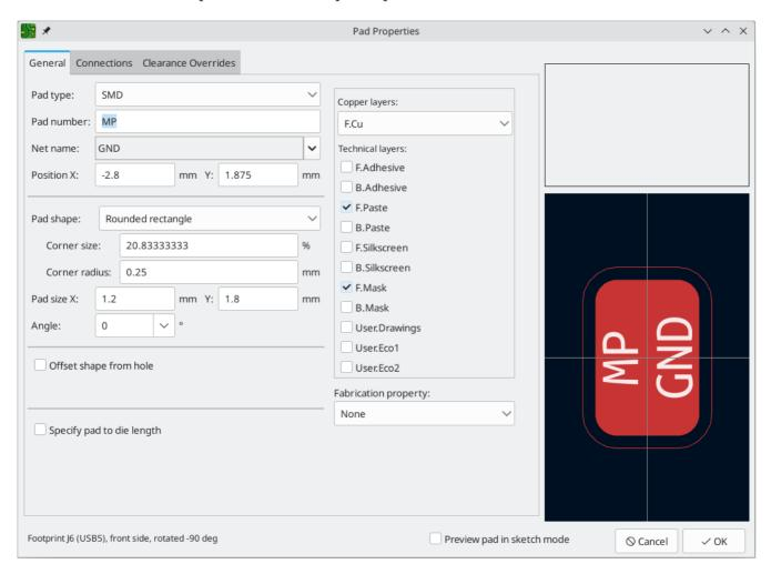
This dialog lets you edit the physical properties of the pad, including size and shape. You can also modify how the pad connects to other objects on the board, including clearance properties, teardrops, and thermal reliefs.
