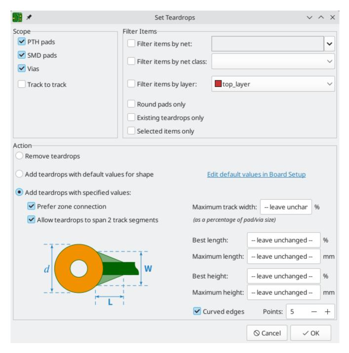
Default properties for teardrops can be configured in the Board Setup dialog. These defaults will be used in the Edit Teardrops dialog when **add teardrops with default values for shape** is selected in that dialog. The defaults are configured separately for teardrops connecting to round shapes, rectangular shapes, or between tracks. The available options for each type of teardrop are the same as in the Edit Teardrops dialog.
