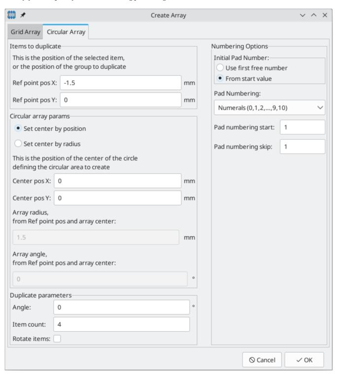
The tool has several options. Pads will be renumbered starting at the selected **first pad number**, and each subsequent pad will have its number incremented by the **numbering step**. You can also choose an optional **pad name prefix** which will be inserted before of the incrementing part of each pad number.
