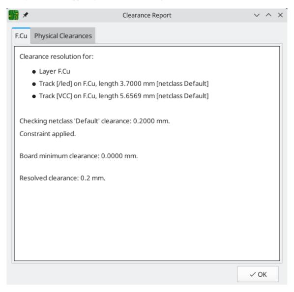
To inspect the design constraints that apply to an object, select it and choose **Constraints Resolution** from the **Inspect** menu. The Constraints Report dialog will show any constraints that apply to the object.
