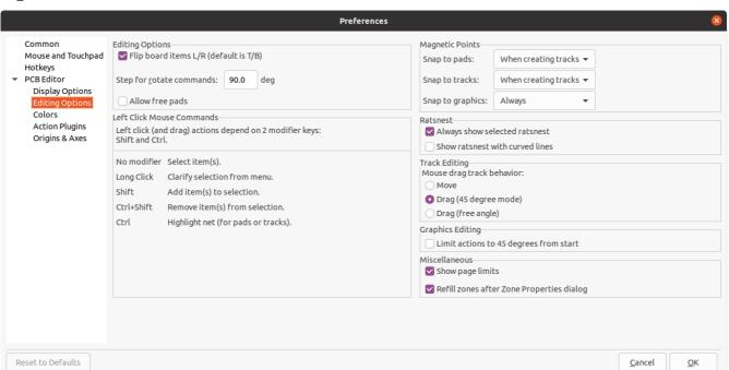
Flip board items L/R: Controls the direction board items will be flipped when moving them between the top and bottom layers. When checked, items are flipped Left-to-Right (about the Vertical axis); when unchecked, items are flipped Top-to-Bottom (about the Horizontal axis).
