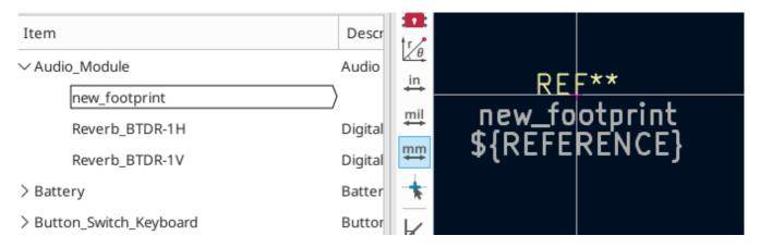
These items are centered on the footprint's anchor (origin point), which is indicated with a magenta cross symbol. The anchor can be repositioned (changing the (0, 0) point for the footprint) by selecting the button and clicking on the new desired anchor position.
