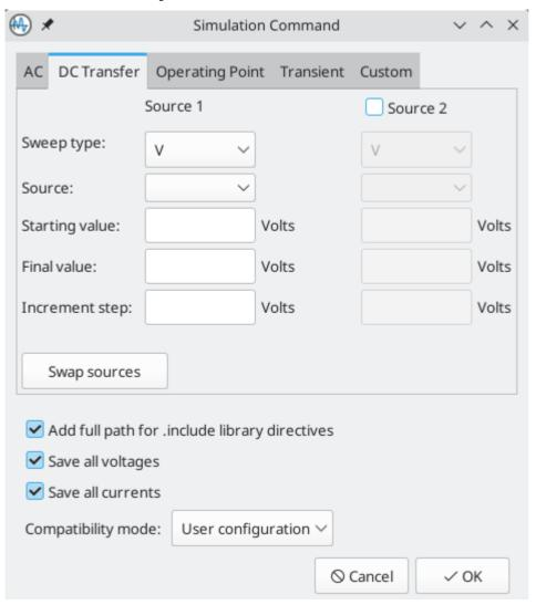
Calculates the DC behavior of the circuit while sweeping one or two parameters: source values (voltage or current), resistor values, or the simulation temperature.
