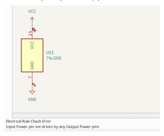
To avoid this warning, connect the net to PWR\_FLAG symbol on such a power net as shown in the following example. The PWR\_FLAG symbol is found in the power symbol library. Alternatively, connect any power output pin to the net; PWR\_FLAG is simply a symbol with a single power output pin.
