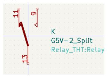
Unit A does not have the same symbol and pin layout as Units B and C, so the units are not interchangeable.
