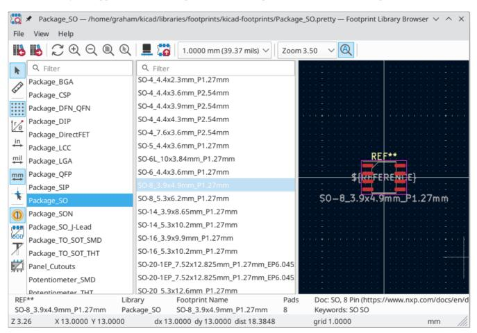
Double clicking the name of a footprint or using the button adds the footprint to the board.
