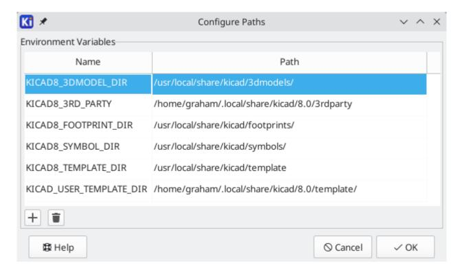
Paths set in the Configure Paths dialog are internal to KiCad and are not visible as environment variables outside of KiCad. They are stored in KiCad's user configuration files.
