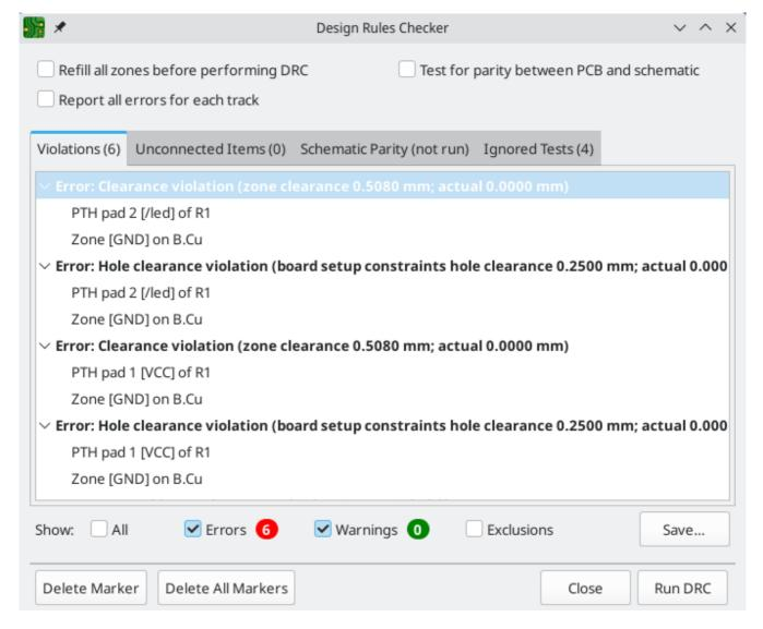
Close the DRC dialog, press B to refill the zone, and re-run DRC. Alternatively, check the **Refill all zones before performing DRC** checkbox and re-run DRC. All violations are fixed.
