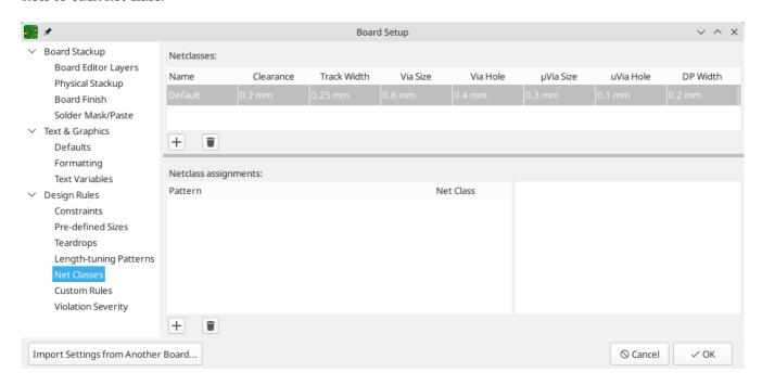
Track width and spacing can be managed manually by the designer during layout, but net classes are recommended because they provide an automatic way to manage and check design rules.
