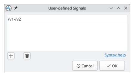
To add a user-defined signal, open the User-defined Signal dialog with **Simulation** → **User-defined Signals...** ( button) and add a signal. The new signal will appear in the Signal grid, where it can be plotted and used like any other signal. User-defined signals are also included in OP results.
