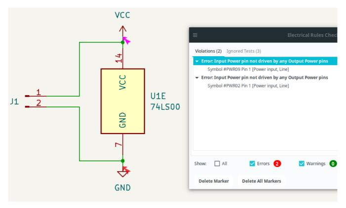
To avoid this warning, connect the net to PWR\_FLAG symbol on such a power net as shown in the following example. The PWR\_FLAG symbol is found in the power symbol library. Alternatively, connect any Output Power pin to the net; PWR\_FLAG is simply a symbol with a single Output Power pin.
