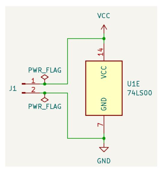
Ground nets often need a PWR\_FLAG to be manually added, even when power rails do not, because voltage regulators have outputs declared as Output Power, but their ground pins are typically marked as Power Inputs. Therefore grounds are not considered driven by these voltage regulators. This is so multiple regulators can share a common ground without errors caused by two Output Power pins being connected together.
