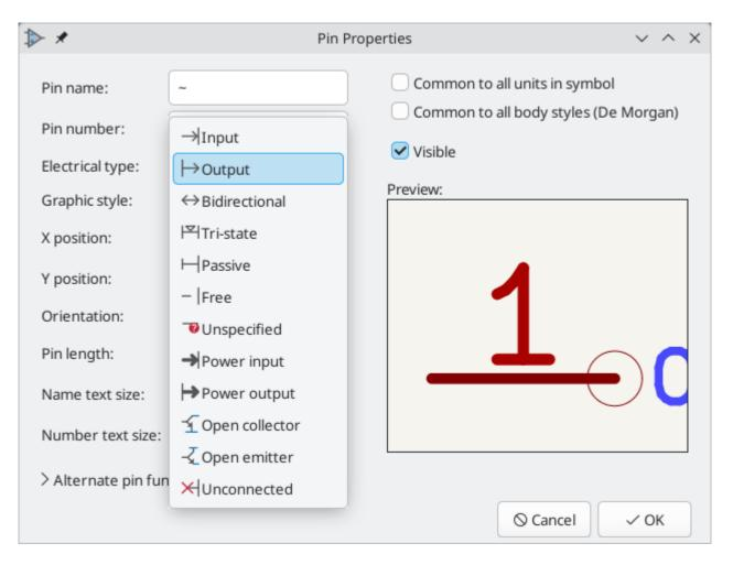
Choosing the correct electrical type is important for the schematic ERC tool. ERC will check that pins are connected appropriately, for example ensuring that input pins are driven and power inputs receive power from an appropriate source.
