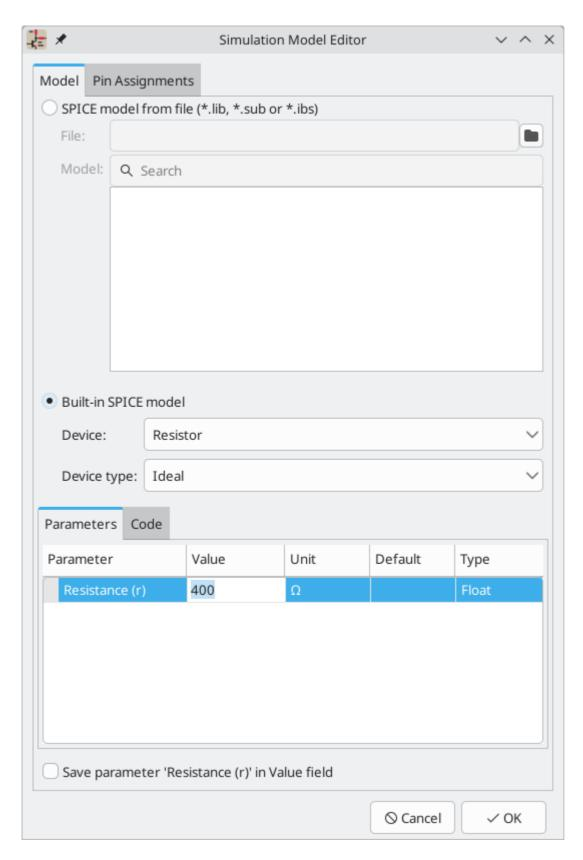
**Device** sets the type of device to simulate: a resistor, BJT, voltage source, etc. This value is stored in the symbol's Sim.Device field.
