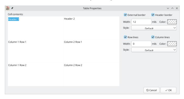
This dialog lets you edit the properties of the entire table, including the text in each cell and the separators between cells. To change the formatting of text in a cell, edit the properties of individual cells, instead of the properties for the entire table.
