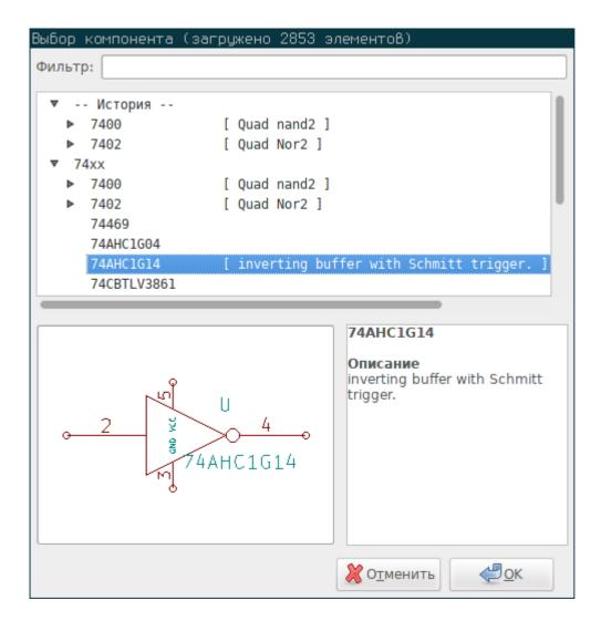
By default, only the symbol/library name and description columns are shown. Additional columns can be added by right-clicking the column header and selecting **Select Columns**.
