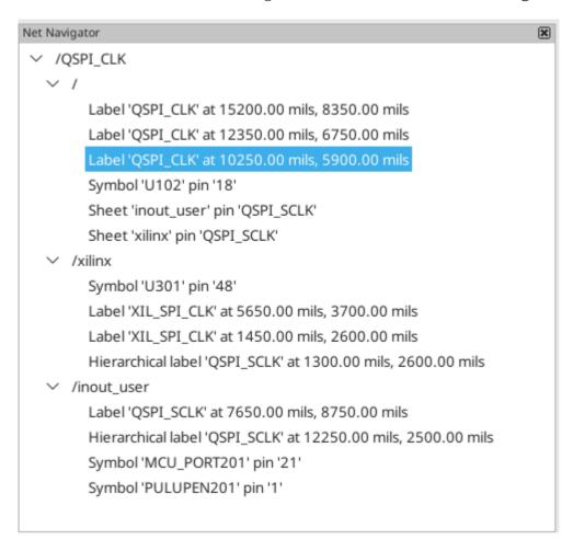
When you highlight a net in the schematic, every place where that net is shown in the schematic is listed in the net navigator panel. All labels, symbol pins, and sheet pins connected to the net are listed. Each occurrence is sorted under its schematic sheet. Clicking on an occurrence displays that item in the editing canvas.
