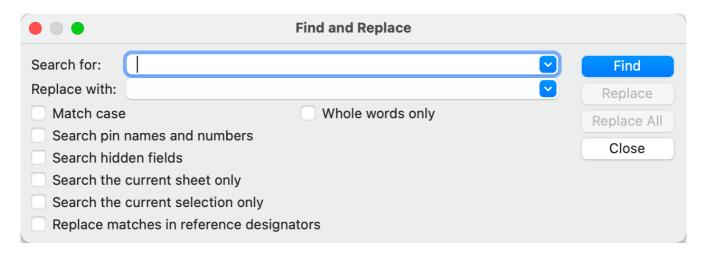
If the **Replace matches in reference designators** option is checked, reference designators will be modified if they contain matching text. Otherwise reference designators will not be affected.
