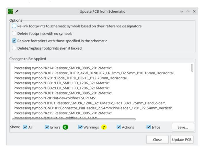
The tool adds the footprint for each symbol to the board and transfers updated schematic information to the board. In particular, the board's net connections are updated to match the schematic. Symbols with the **Exclude from board** attribute are not transferred to the PCB.
