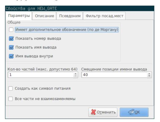
It is important to set the **number of units** and check **all units are interchangeable** and **has alternate body style**, as applicable, because these settings affect how pins and graphics are added to each symbol unit.
