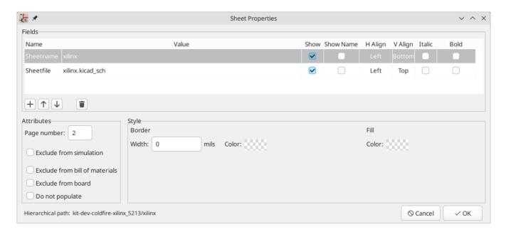
The **sheet name** must be unique, as it is used in the full net name for any nets in the subsheet. For example, a net with the local label net1 in the sheet sheet1 would have a full net name of /sheet1/net1. The sheet name is also used to refer to the sheet in various places in the GUI, including the title block and the hierarchy navigator. The sheet name can also be changed in the hierarchy navigator.
