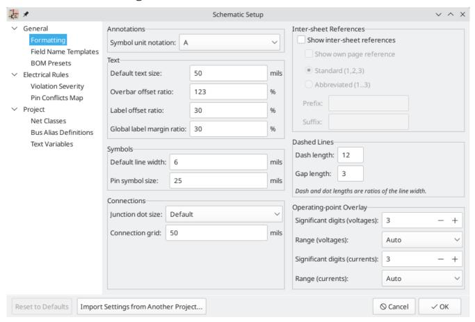
The formatting panel contains settings for the appearance of symbols, text, labels, graphics, and wires.
