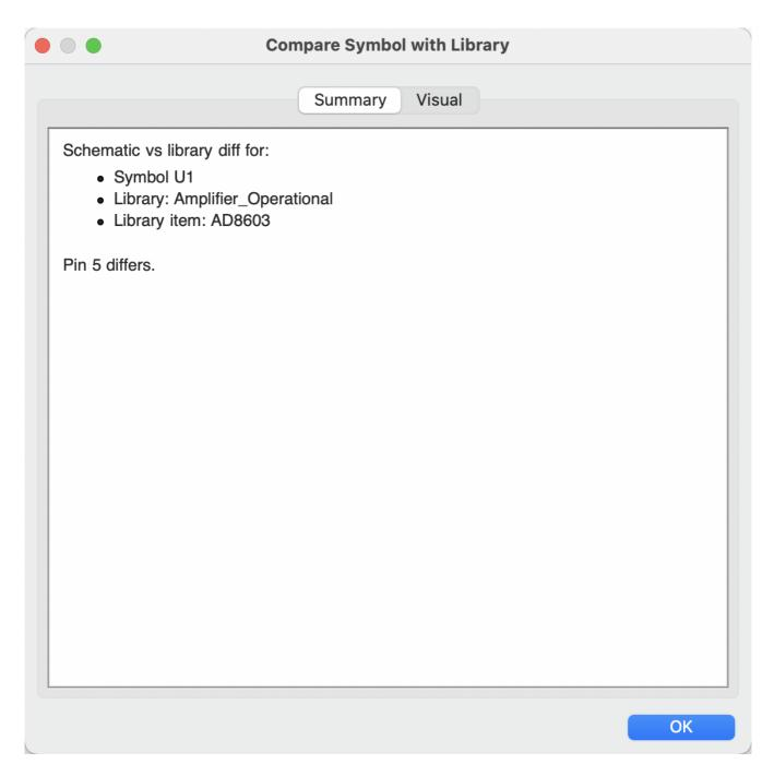
The **Summary** tab shows the name of the symbol, including its library and schematic reference designator, and provides a list of the differences between the schematic and library versions of the symbol.
