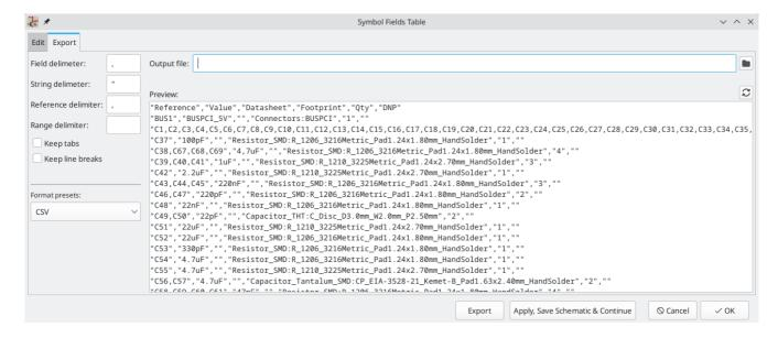
At the top you can specify the output file. Pressing the **Export** button will write the BOM to this file path. This path can contain text variables.
