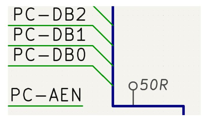
Directive labels are added with the **QA** button in the right toolbar. They behave like labels, except that they cannot be used to name a net. The attached net is assigned a net class according to the value of the directive's Net Class field. The Net Class field presents a dropdown list of all the net classes that have been specified in Schematic Setup or Board Setup.
