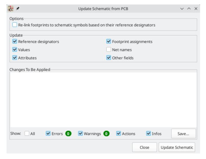
The tool syncs changes in reference designators, values, attributes (like DNP or Exclude From BOM), footprint assignments, other fields, and net names from the board to the schematic. Each type of change can be individually enabled or disabled.
