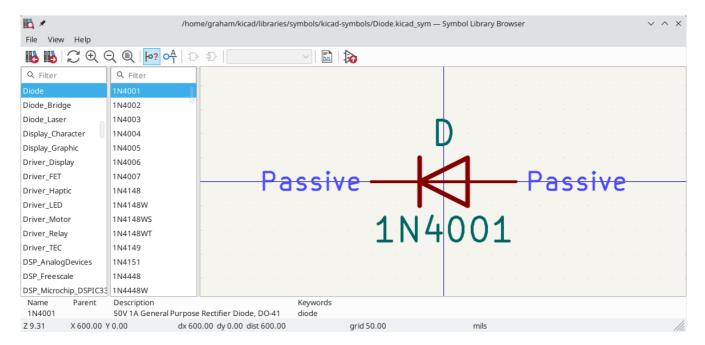
Double clicking the name of a symbol or using the houtenadds the symbol to the schematic.
