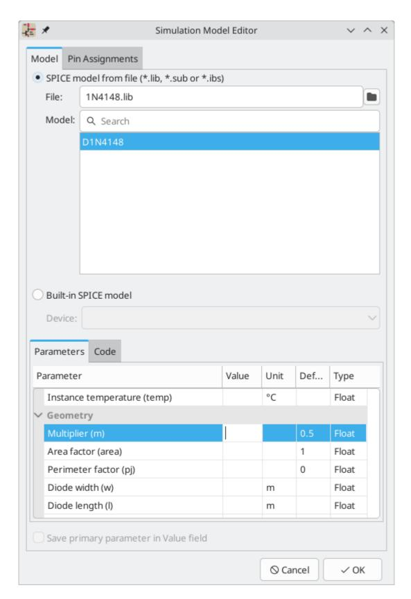
**File** is the path to the model file to use. Unencrypted model files are plain, human-readable text files and often have extensions such as .lib, .sub etc., although KiCad will accept a valid model with any extension.
