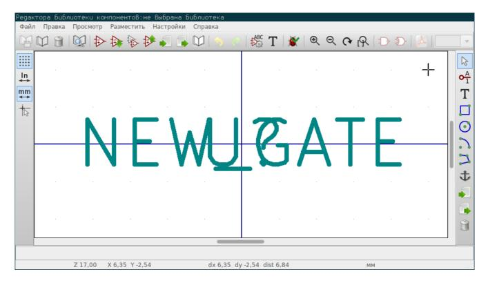
The blue cross in the center is the symbol anchor, which specifies the symbol origin i.e. the coordinates (0, 0). The anchor can be repositioned by selecting the \* button and clicking on the new desired anchor position.
