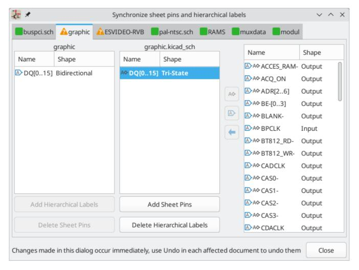
This dialog shows the hierarchical labels and hierarchical sheet pins for each hierarchical sheet. If the tool was launched from the context menu of a sheet symbol, only one tab will be available, with the labels and sheet pins for that specific sheet. If the tool was started globally, i.e. with the button or with **Place** → **Sync Sheet Pins**, a tab will be shown for each hierarchical sheet.
