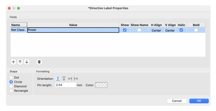
In addition to the associated net class, you can edit the directive's **shape** (dot, circle, diamond, or rectangle), **orientation**, **pin length**, and **color** in the directive's properties.
