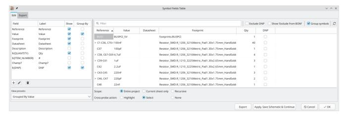
Fields with the **Show** box checked will be included as columns in the BOM, and fields with the **Group By** box checked are used to group components together. Components are grouped into the same line if all of their **Group By** fields are identical and the **Group symbols** box is checked. You can set an arbitrary column name for each field and reorder columns by dragging their headers.
