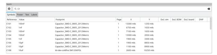
You can optionally filter the list based on a search string. When no filter is used, all items in the design are listed in the corresponding tab. Items from the entire schematic are listed, not just items in the current sheet. Items are filtered based on their properties:
