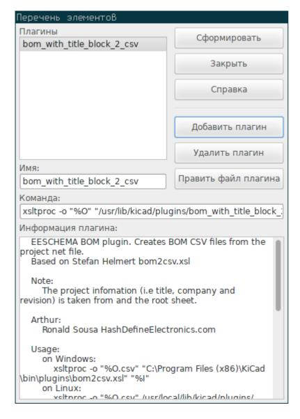
Several BOM generator scripts are included with KiCad, and users can also create their own. BOM generator scripts generally use Python or XSLT, but other tools can be used as long as you can specify a command line for KiCad to execute when running the generator.
