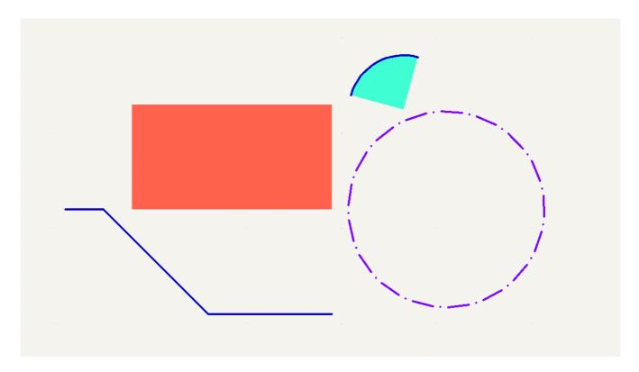
Line width, color, and style (solid, dashed, or dotted) can be configured in the properties dialog for each shape (E). Rectangles, circles, and arcs can also have a fill color set and have their outlines removed.
