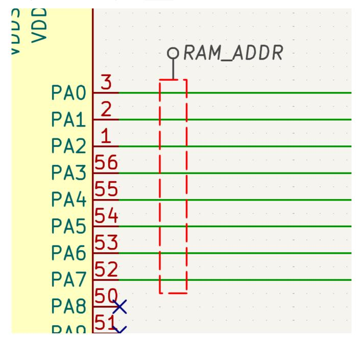
You can show or hide directive labels in the schematic using the **View** → **Show Directive Labels** option.
