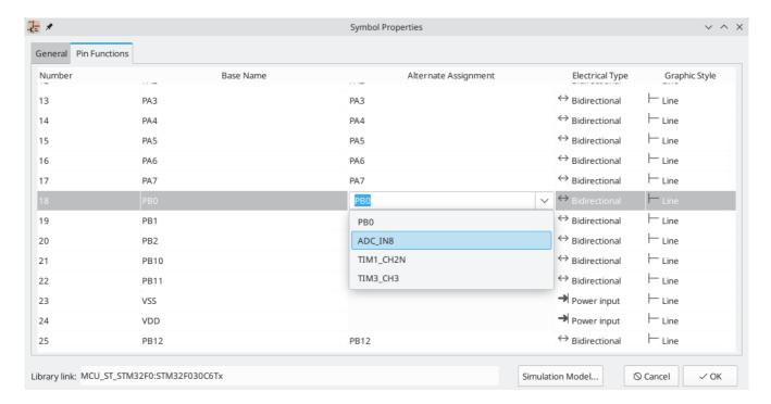
Pins that have alternate functions available are displayed with a small graphical indicator next to the pin name, as shown in the screenshot below. To globally show or hide these indicators, use  $View \rightarrow Show Pin$  Alternate Icons.
