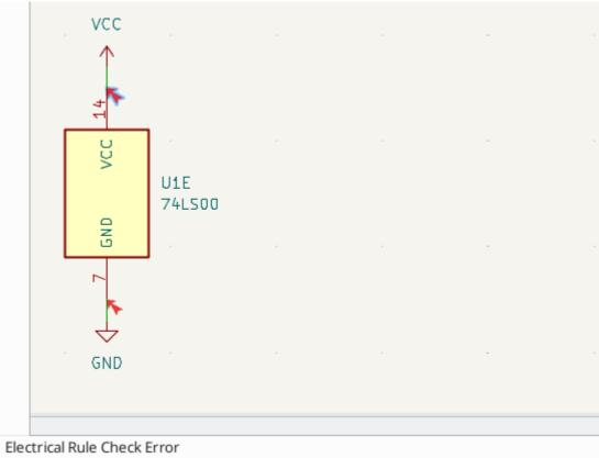
Input Power pin not driven by any Output Power pins
