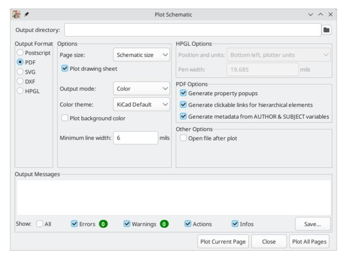
The **Output Messages** pane displays messages about the generated files. Different kinds of messages can be shown or hidden using the checkboxes, and the messages can be saved to a file using the **Save...** button.
