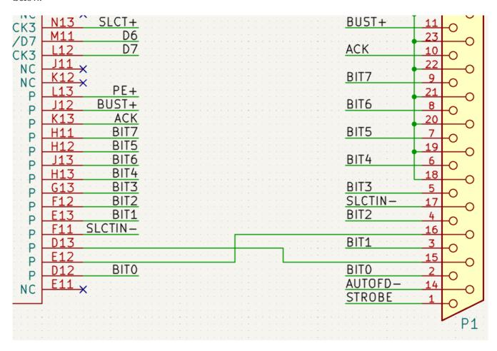
Connections can also be made with buses and with implicit connections via hidden power pins.
