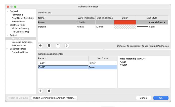
The top pane lists the net classes that exist in the design. The Default net class always exists, and you can add additional net classes with the + button or remove the selected net class with the = button.
