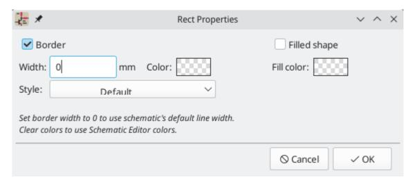
Setting a shape's line width to 0 uses the schematic default line width, which is configurable in Schematic Setup. Spacing for line dashes is also configurable there. Removing a line or fill color uses the color theme's graphics color, which is configurable in Preferences.
