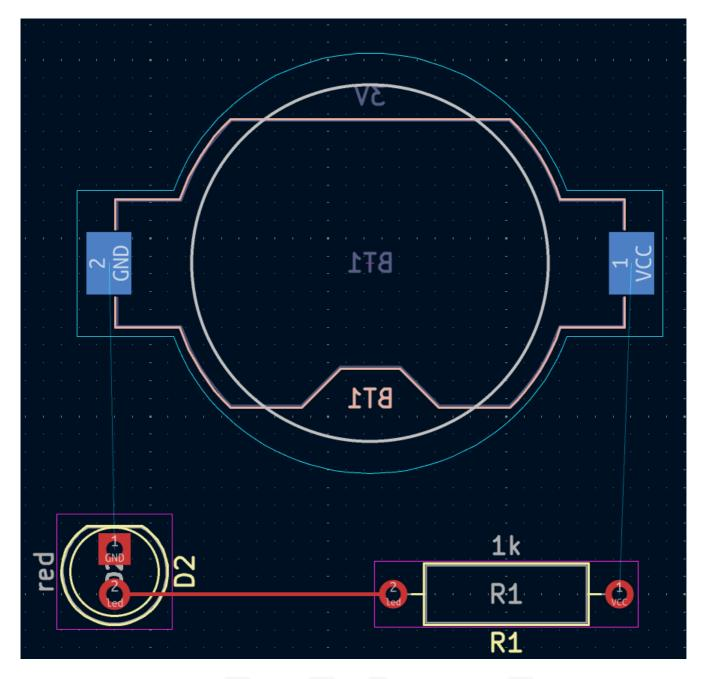
Now draw a track between the GND pads of BT1 and D1, starting with the BT1 pad on the back of the board. Notice that the active layer automatically changed to B.Cu after clicking on the BT1 pad. Click on the D1 pad to finish the track.
