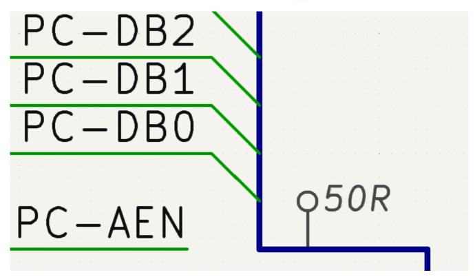
Directive labels are added with the  $\mathbf{Q}\mathbf{A}$  button in the right toolbar. They behave like labels, except that they cannot be used to name a net. The attached net is assigned a net class according to the value of the directive's
