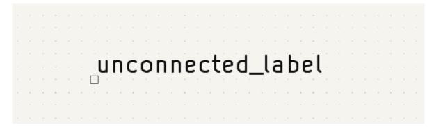
The connection point's position relative to the label text can be changed by choosing a different label orientation in the label's properties, or by mirroring/rotating the label.
