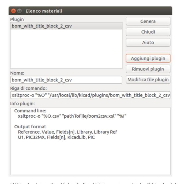
Additional scripts can be added to the list of BOM generator scripts by clicking the + button. Scripts can be removed by clicking the  $\uparrow$  button. The  $\nearrow$  button opens the selected script in a text editor.
