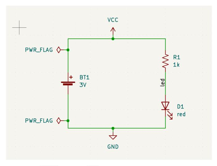
There is a special PWR\_FLAG symbol in the Power symbol library that is used to solve this problem by telling KiCad that the nets are actually driven. Add this symbol to the VCC and GND nets and re-run ERC. When ERC passes without any violations, the schematic is complete.
