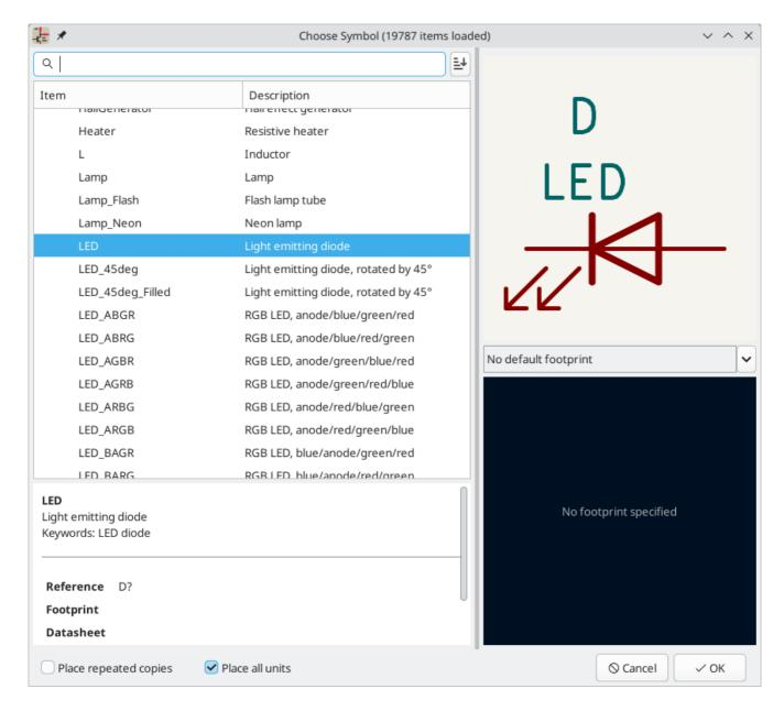
Next, add a current-limiting resistor. Go back to the symbol chooser, but this time try searching for a resistor by entering R in the filter box at the top. Again, it is found in the Device library. The R device is an IEC-style rectangular resistor symbol. An R\_US symbol is also available for users who prefer the ANSI-style zigzag symbol. Select a resistor symbol and add it to the schematic.
