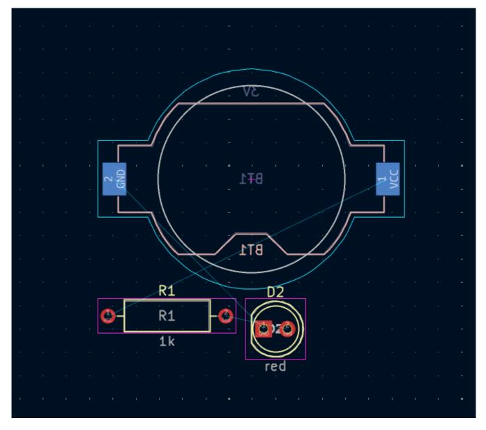
All PCB layers are viewed from front side of the board. Footprints on the bottom of the board are therefore upside down and appear mirrored.
