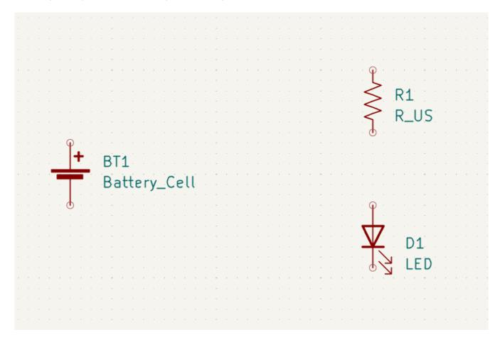
In KiCad, objects are selected by clicking on them while the selection tool is active. The selection tool is the default tool when no other tool is active, so you can enter the selection tool by quitting any active tool (Esc) or by clicking the k button in the right toolbar.
