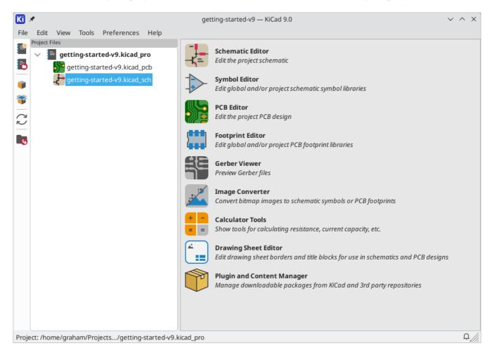
At left, the Project Files pane lists the files in the new project. There is a project file with the extension .kicad\_pro, a schematic file with the extension .kicad\_sch, and a board file with the extension .kicad\_pcb. These files all share a name with your project.
