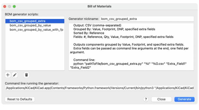
Several BOM generator scripts are included with KiCad, and users can also create their own. BOM generator scripts generally use Python or XSLT, but other tools can be used as long as you can specify a command line for KiCad to execute when running the generator.
