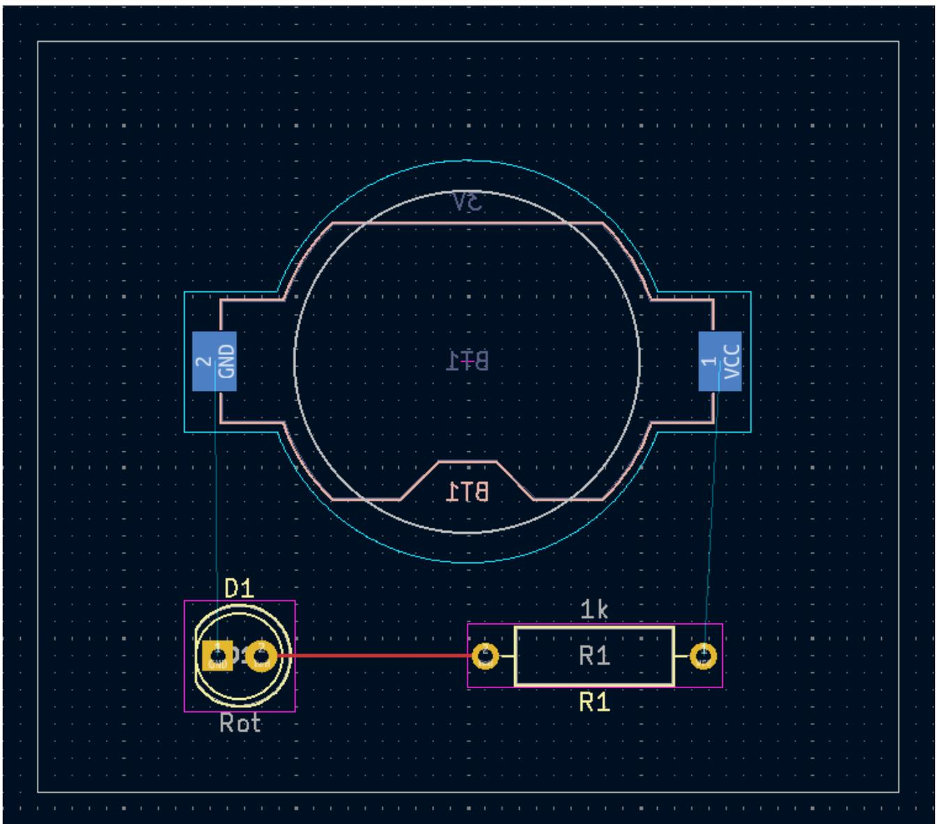
Now draw a track between the GND pads of BT1 and D1, starting with the BT1 pad on the back of the board. Notice that the active layer automatically changed to B.Cu after clicking on the BT1 pad. Click on the D1 pad to finish the track.
