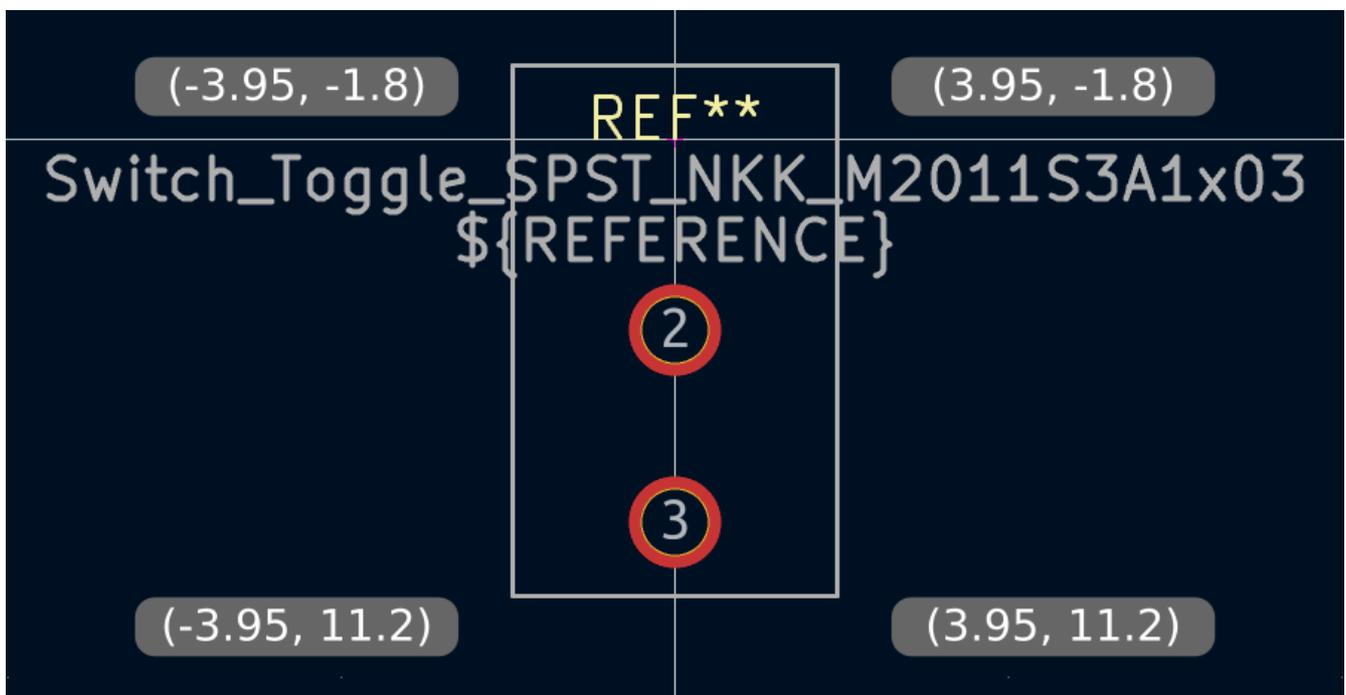
Next, switch to the F.Silkscreen layer. We want the silkscreen outline to be just outside of the part outline, so the silkscreen lines will be drawn 0.11 mm to the outside of the lines on the fabrication layer (0.11 mm is half of the 0.10 mm fab line width, plus half of the 0.12 mm silkscreen line width). The exact coordinates are shown in the screenshot below, and helpful grid settings are:
