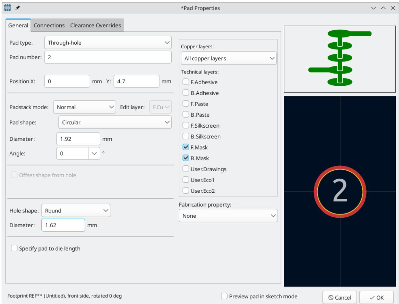
Now use the **Add a pad** tool again to place the other pad at (0, 9.4 mm). Notice that the pad number is automatically incremented and the properties including pad size and hole size are copied from the previous pad.
