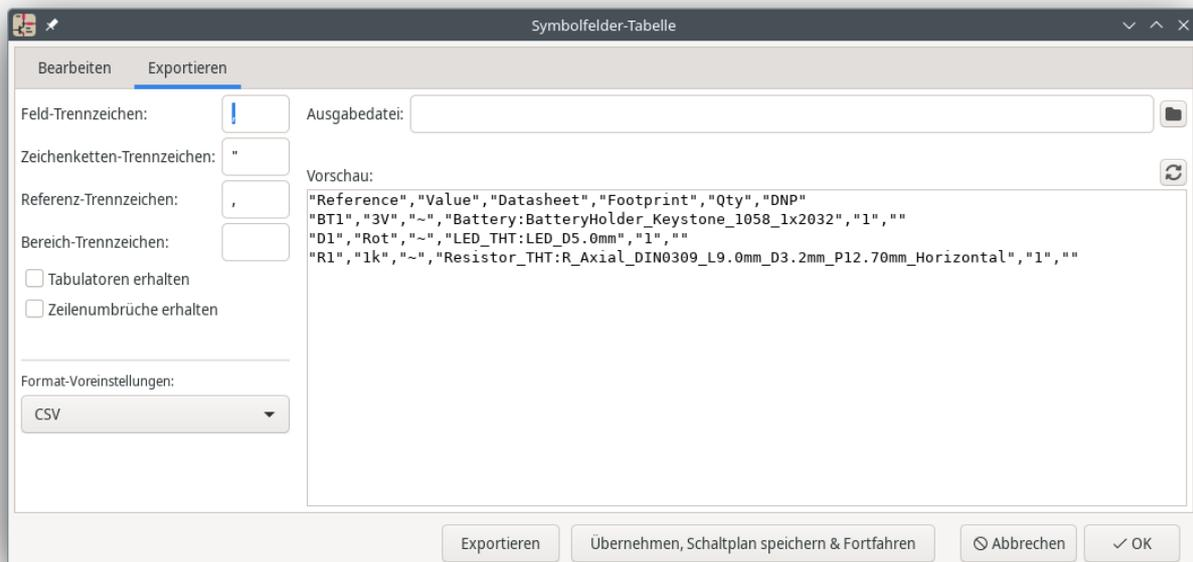
KiCad has a GUI for BOM export. You can configure which symbol metadata will be exported, and how the symbols are grouped, in the **Edit** tab, and configure the output format in the **Export** tab.
