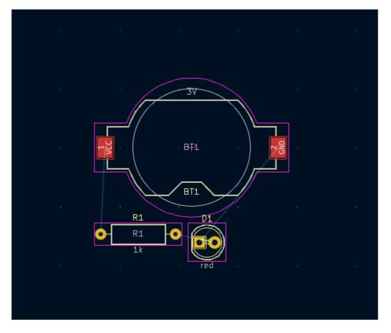
In KiCad, updating the PCB with changes in the schematic is a manual process: the designer decides when it is appropriate to update the PCB with modifications in the schematic. Each time the schematic is edited, the designer must use the **Update PCB from Schematic** tool to keep the schematic and layout in sync.
