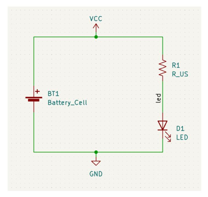
Note that labels and power symbols with the same name are connected together. Another GND symbol or wire labeled led on this schematic page would be shorted to the existing one, even without wires visually connecting them.
