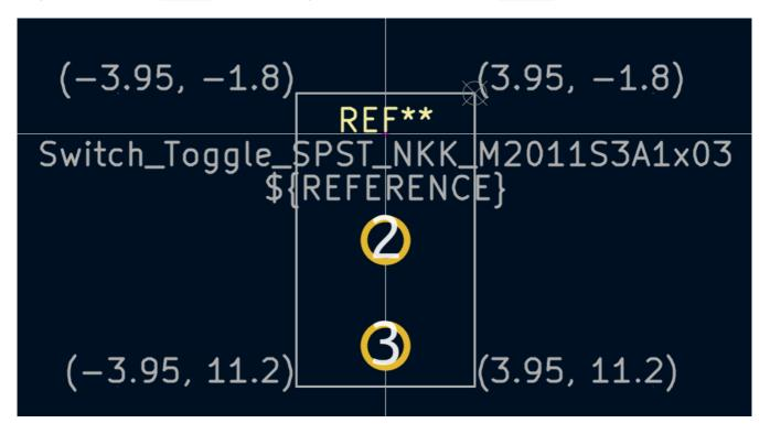
Next, switch to the F.Silkscreen layer. We want the silkscreen outline to be just outside of the part outline, so the silkscreen lines will be drawn 0.11 mm to the outside of the lines on the fabrication layer (0.11 mm is half of the 0.10 mm fab line width, plus half of the 0.12 mm silkscreen line width). The exact coordinates are shown in the screenshot below, and helpful grid settings are:
