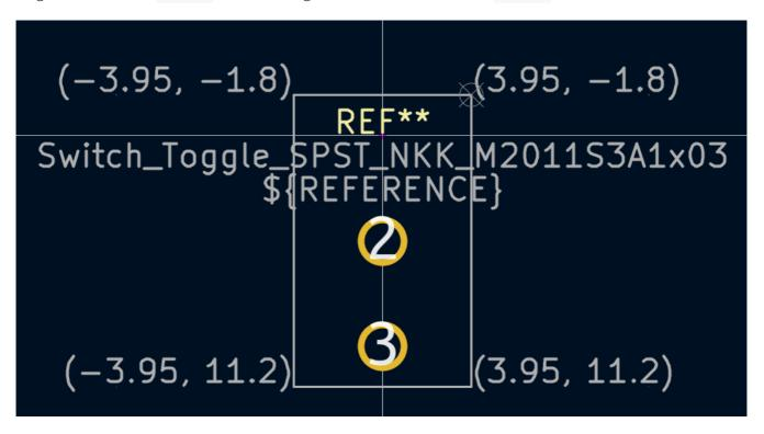
Next, switch to the F.Silkscreen layer. The silkscreen outline should be just outside of the part outline, so the silkscreen lines are moved outwards from the fabrication drawing by 0.11 mm (half of 0.10 mm fab line width, plus half of the 0.12 mm silkscreen line width). The exact coordinates are shown in the screenshot below, and helpful grid settings are:
