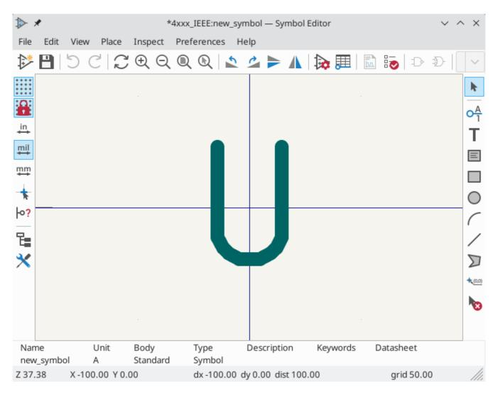
The blue cross in the center is the symbol anchor, which specifies the symbol origin i.e. the coordinates (0, 0). The anchor can be repositioned by selecting the specifies the symbol and clicking on the new desired anchor position.
