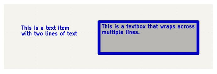
Both kinds of text item support multiline text and basic formatting features, but text boxes wrap text to fit in the outline and have additional formatting options. All text has adjustable fonts, color, size, bold and italic emphasis, left and right alignment, and vertical and horizontal orientation. Text boxes additionally support horizontal centering, vertical alignment options, and colored borders and fill. NOTE
