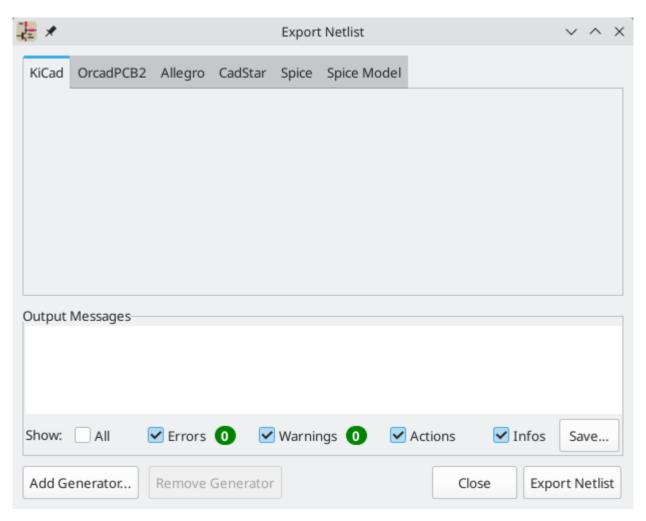
KiCad supports exporting netlists in several formats: KiCad, OrcadPCB2, CADSTAR, Spice, and Spice Model. Each format can be selected by selecting the corresponding tab at the top of the window. Some netlist formats have additional options.
