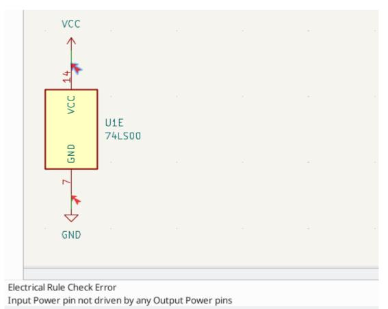
Ground nets often need a PWR\_FLAG as well, because voltage regulators have outputs declared as power outputs, but their ground pins are typically marked as power inputs. Therefore grounds can appear unconnected to a source unless a PWR\_FLAG symbol is used.
