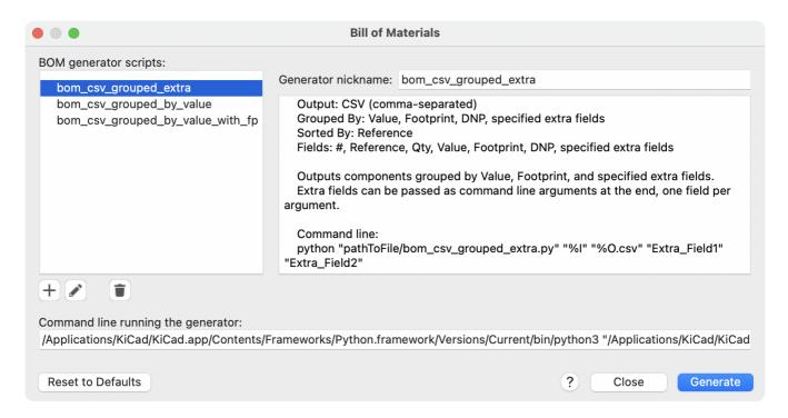
Additional scripts can be added to the list of BOM generator scripts by clicking the + button. Scripts can be removed by clicking the  $\stackrel{\bullet}{\blacksquare}$  button. The  $\stackrel{\bullet}{\triangleright}$  button opens the selected script in a text editor.
