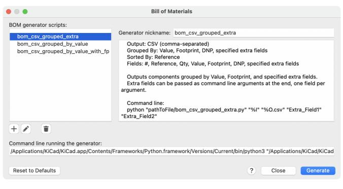
Additional scripts can be added to the list of BOM generator scripts by clicking the + button. Scripts can be removed by clicking the i button. The state of button opens the selected script in a text editor.
