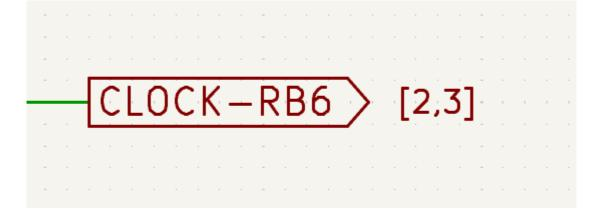
A Sheet References field with value \${INTERSHEET\_REFS} is automatically added to global labels, and is used to control the appearance of inter-sheet references for that label. The \${INTERSHEET\_REFS} text
