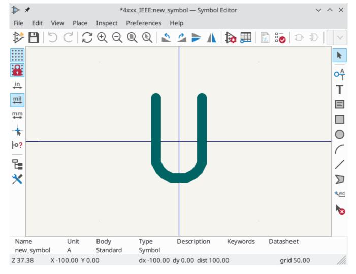
The blue cross in the center is the symbol anchor, which specifies the symbol origin i.e. the coordinates (0, 0). The anchor can be repositioned by selecting the \* icon and clicking on the new desired anchor position.
