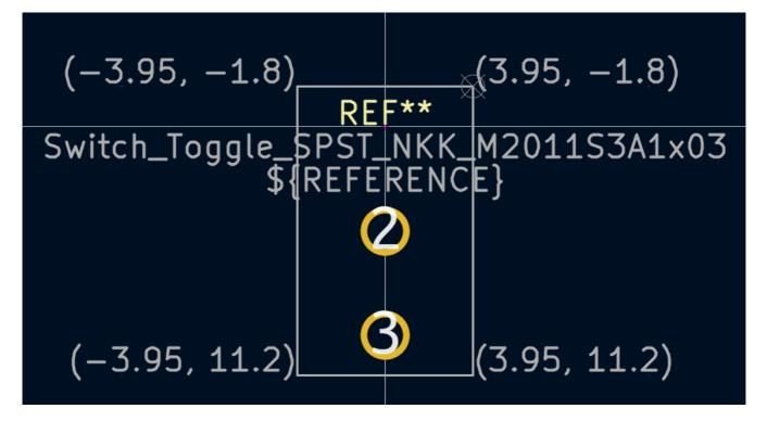
Next, switch to the F.Silkscreen layer. The silkscreen outline should be just outside of the part outline, so the silkscreen lines are moved outwards from the fabrication drawing by 0.11 mm (half of 0.10 mm fab line width, plus half of the 0.12 mm silkscreen line width). The exact coordinates are shown in the screenshot below, and helpful grid settings are:
