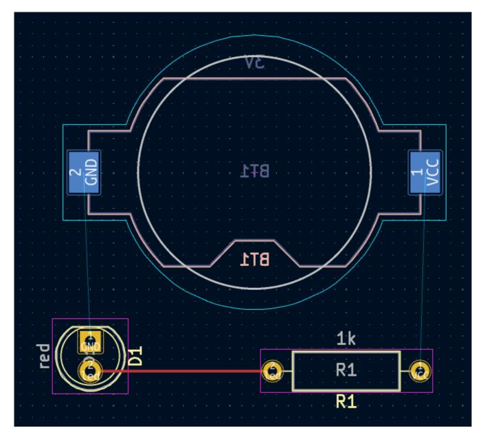
Now draw a trace between the GND pads of BT1 and D1, starting with the BT1 pad on the back of the board. Notice that the active layer automatically changed to B.Cu after clicking on the BT1 pad. Click on the D1 pad to finish the track.
