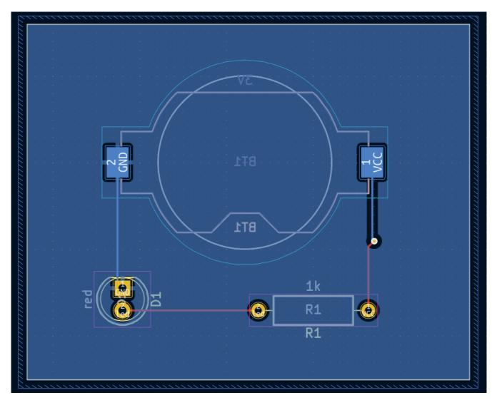
In KiCad, zones are not filled automatically when they are first drawn or modified, or when footprints within them are moved. Zones are refilled by manually filling them and when running DRC. Make sure zone fills are up-to-date before generating fabrication outputs.
