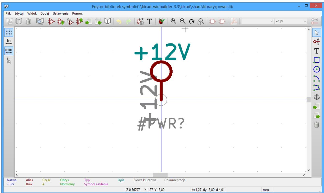
Power symbols consist of a pin of type "Power input" that is marked invisible. They must also have the **Define as power symbol** property checked. [Invisible power input pins](#) have a special property of making implicit global connections based on the pin name.
