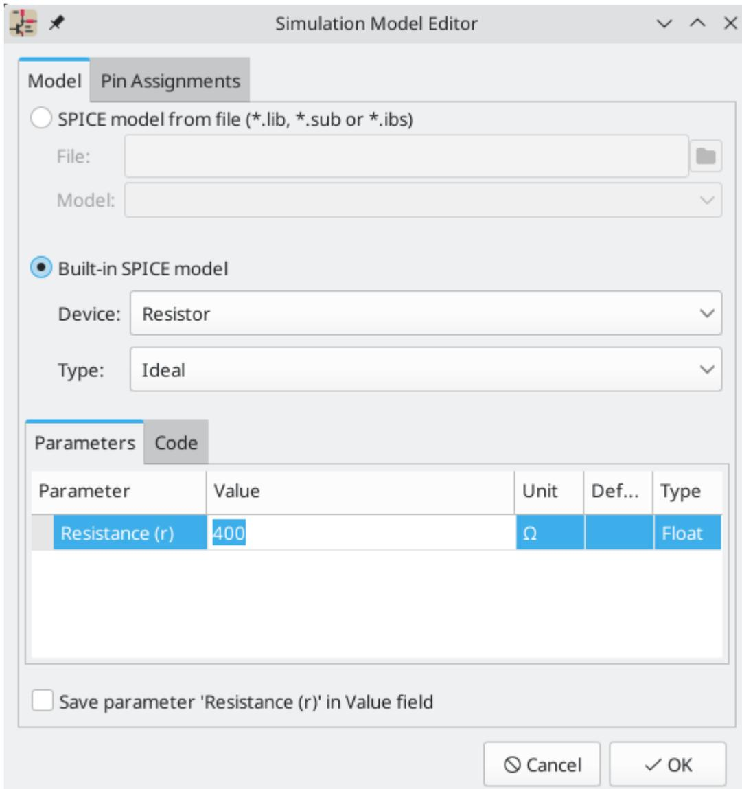
**Device** sets the type of device to simulate: a resistor, BJT, voltage source, etc. This value is stored in the symbol's `Sim.Device` field.
