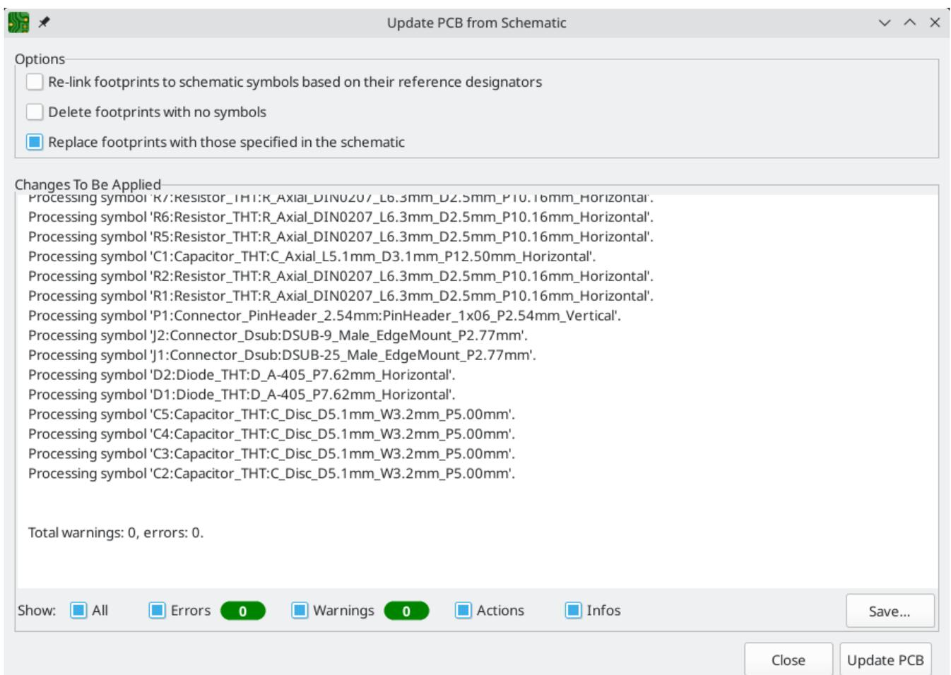
The tool adds the footprint for each symbol to the board and transfers updated schematic information to the board. In particular, the board's net connections are updated to match the schematic. Symbols with the [Exclude from board attribute](#) are not transferred to the PCB.
