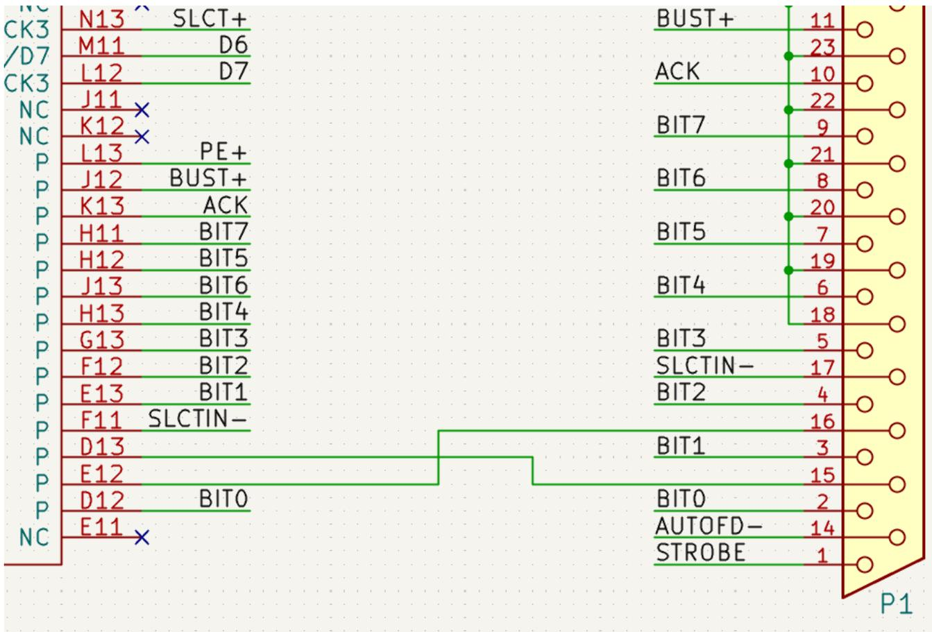
Connections can also be made with buses and with implicit connections via hidden power pins.
