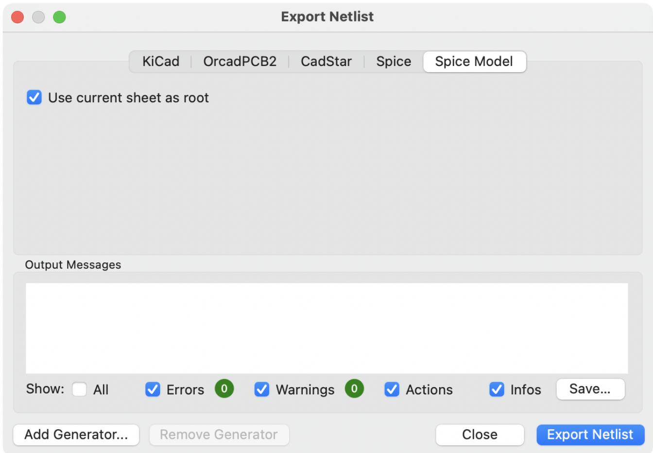
KiCad can also export a netlist of the schematic as a Spice subcircuit model, which can be included in a separate Spice simulation. Any hierarchical labels in the schematic are used as pins for the subcircuit model. Each pin in the model is annotated with a comment describing the pin's electrical direction:
