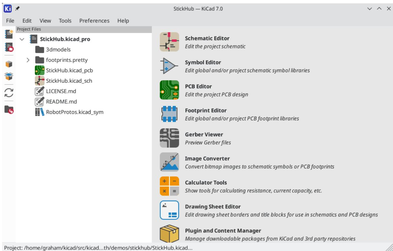
The KiCad project manager window is composed of a tree view on the left showing the files associated with the open project, and a launcher on the right containing shortcuts to the various editors and tools.
