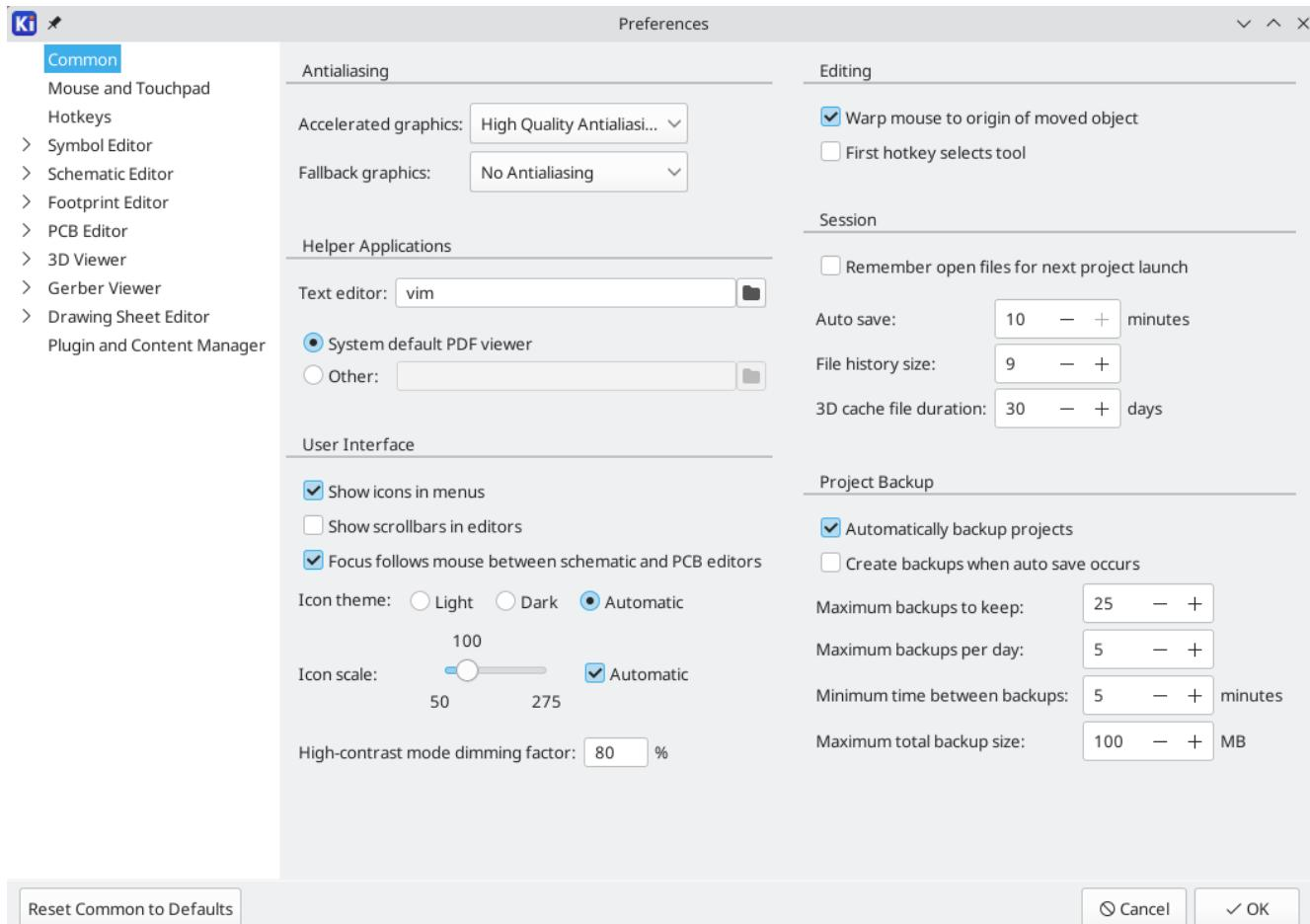
**Accelerated graphics antialiasing:** KiCad can use different methods to prevent aliasing (jagged lines) when rendering using a graphics card. Different methods may look better on different hardware, so you may want to experiment to find the one that looks best to you.
