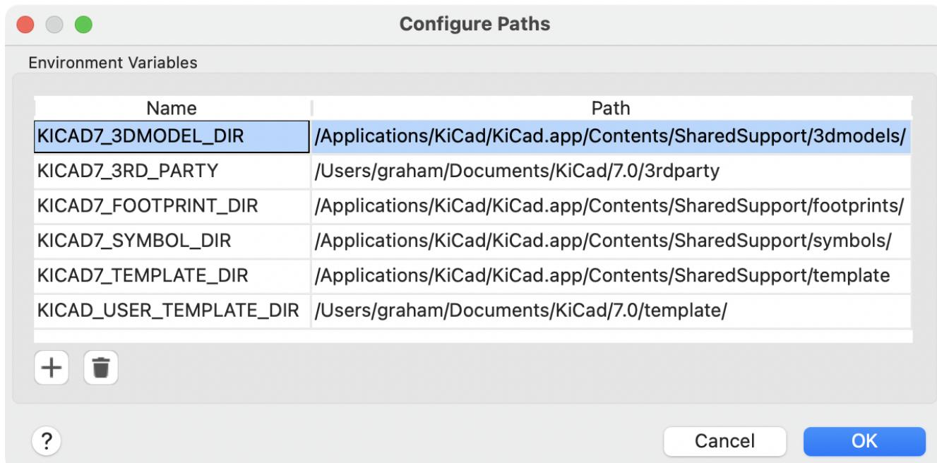
Paths set in the Configure Paths dialog are internal to KiCad and are not visible as environment variables outside of KiCad. They are stored in [KiCad's user configuration files](#).
