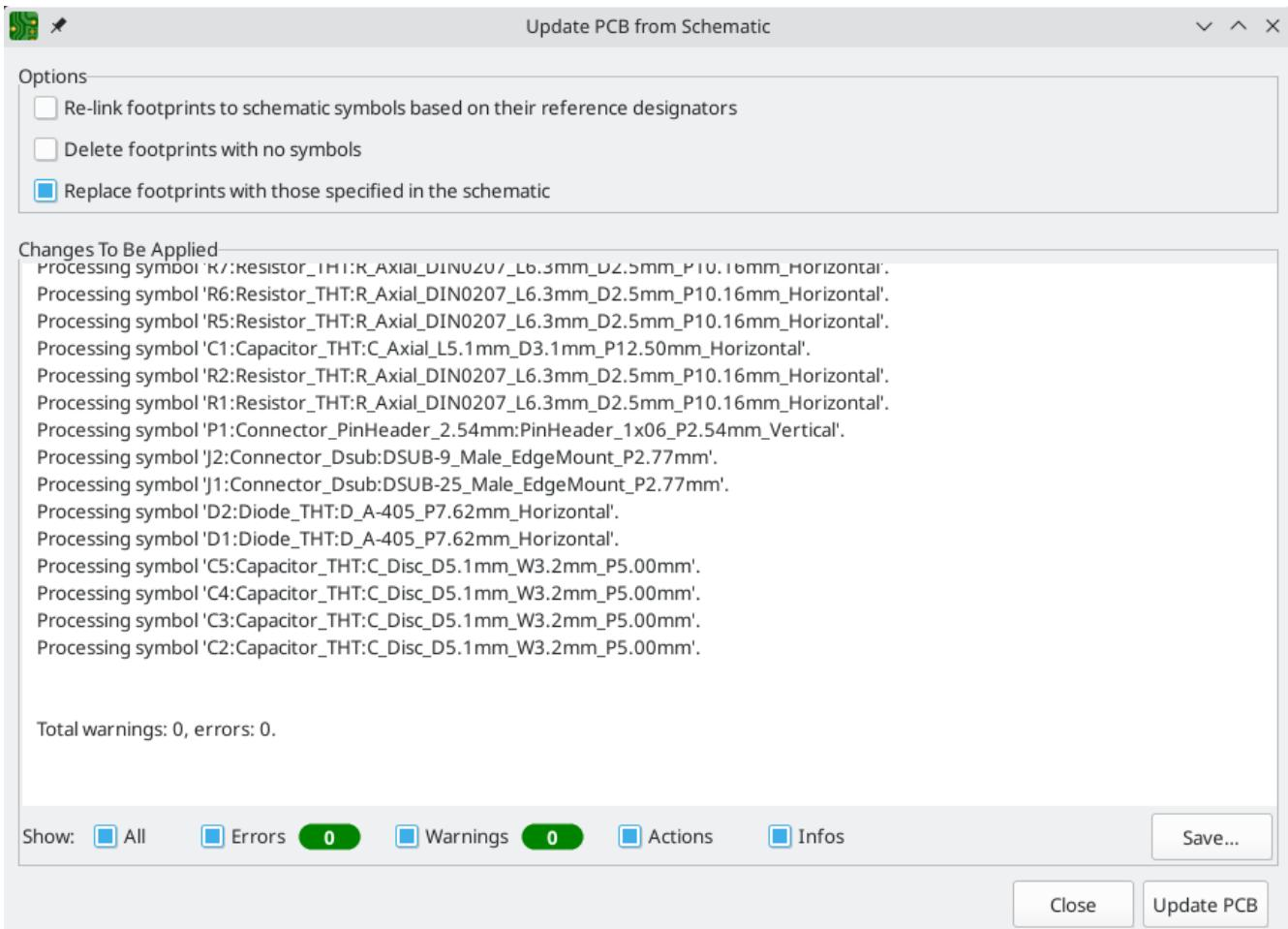
The tool adds the footprint for each symbol to the board and transfers updated schematic information to the board. In particular, the board's net connections are updated to match the schematic.
