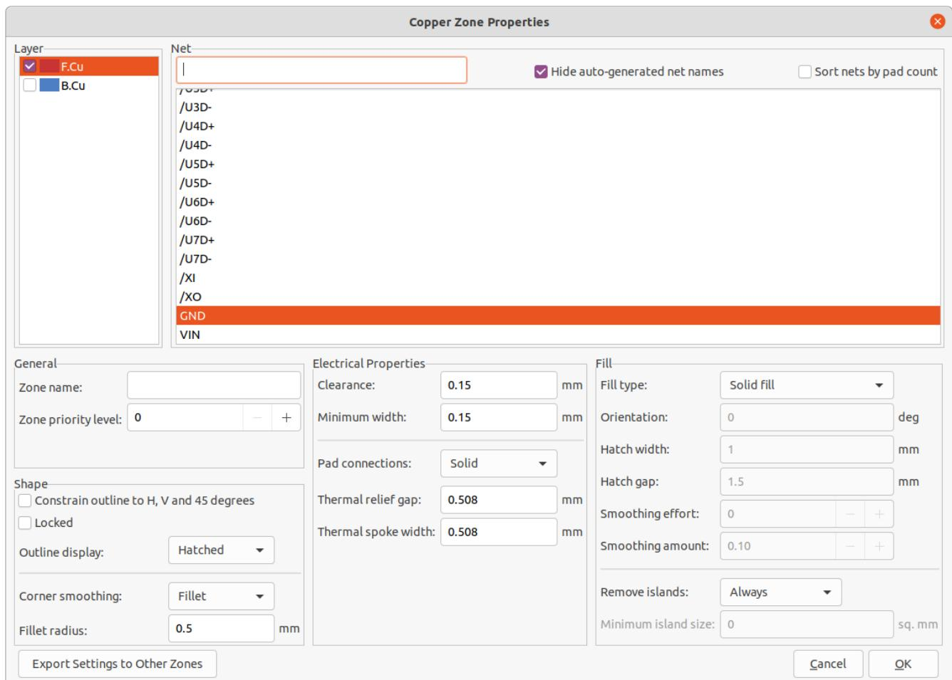
**Layer:** A single zone object can create filled copper on one or more copper layers. Check the box next to each copper layer that this zone outline should fill on. The copper on each layer will be filled independently, but all layers will share the same net.
