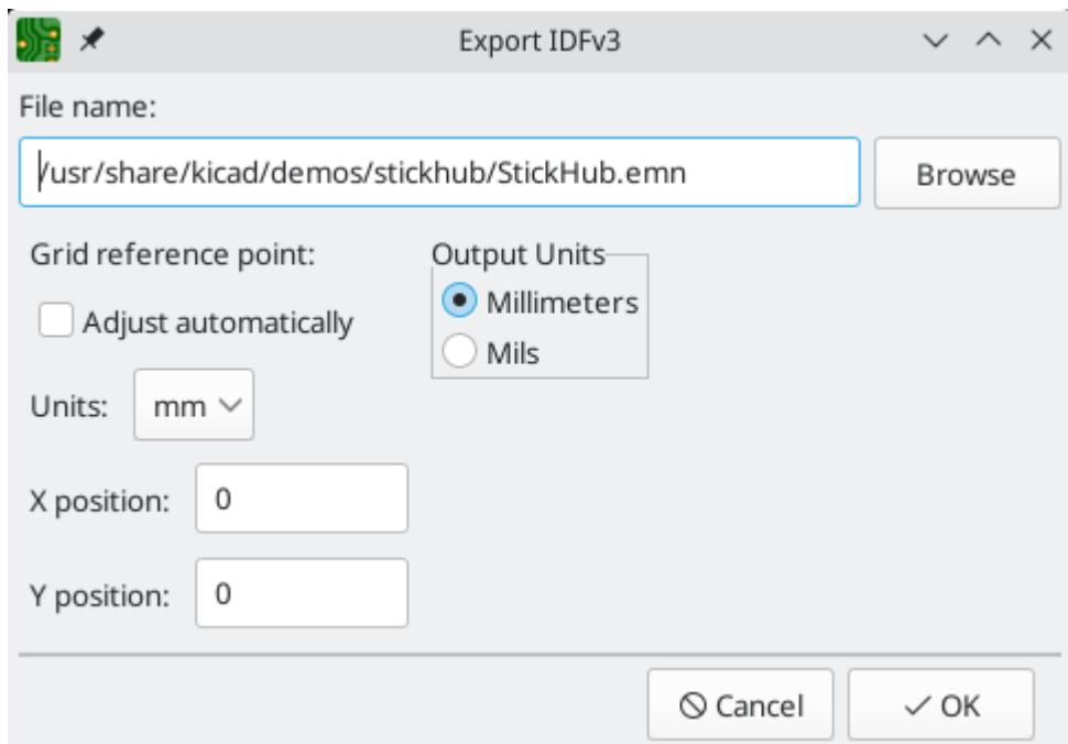
**Grid reference point:** Choose where the exported model's reference point should be. If the **Adjust automatically** option is selected, KiCad will set the reference point to the centroid of the PCB. Otherwise, the reference point is set relative to the display origin.
