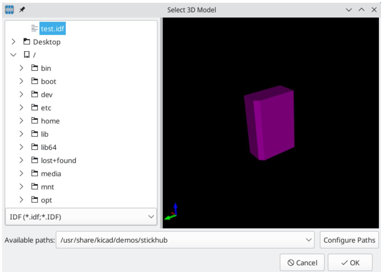
Once the desired component outline file is selected, enter any necessary values for the offset and rotation. The offsets must be specified using the IDF board output units (mm or mils) and in the IDF coordinate system, which is a right-hand coordinate system with +Z pointing towards the viewer, +X to the viewer's right, and +Y towards the upper edge of the screen. The rotation must be in degrees; positive rotation is a counter-clockwise rotation as described in the IDFv3 specification.
