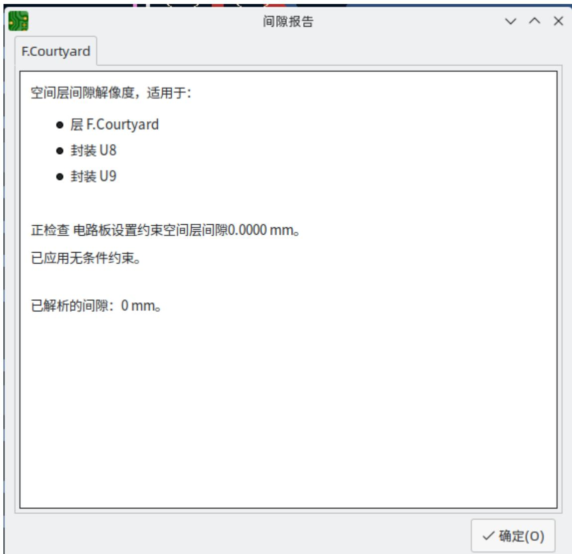
To inspect the design constraints that apply to an object, select it and choose Constraints Resolution from the Inspect menu. The Constraints Report dialog will show any constraints that apply to the object.
