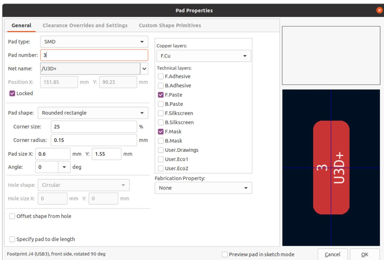
The General tab of the pad properties dialog shows the physical properties of the pad, including its geometry, shape, and layer settings.
