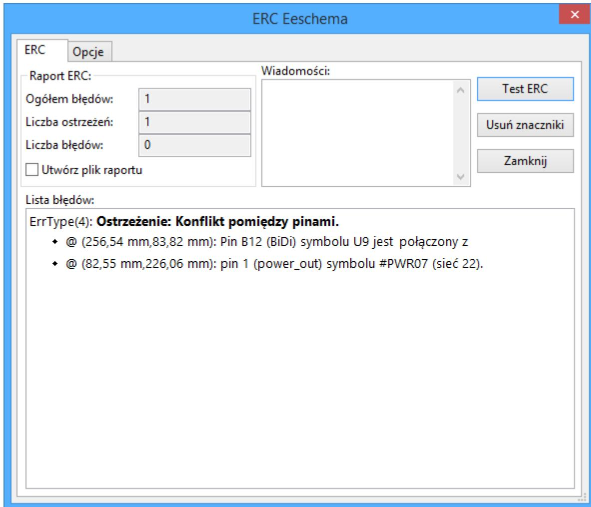
Any warnings or errors are reported in the **Violations** tab, and markers for each violation are placed in the schematic so that they point to the relevant part of the schematic. Warnings are indicated by yellow arrows, and errors have red arrows. Excluded violations are shown as green arrows.
