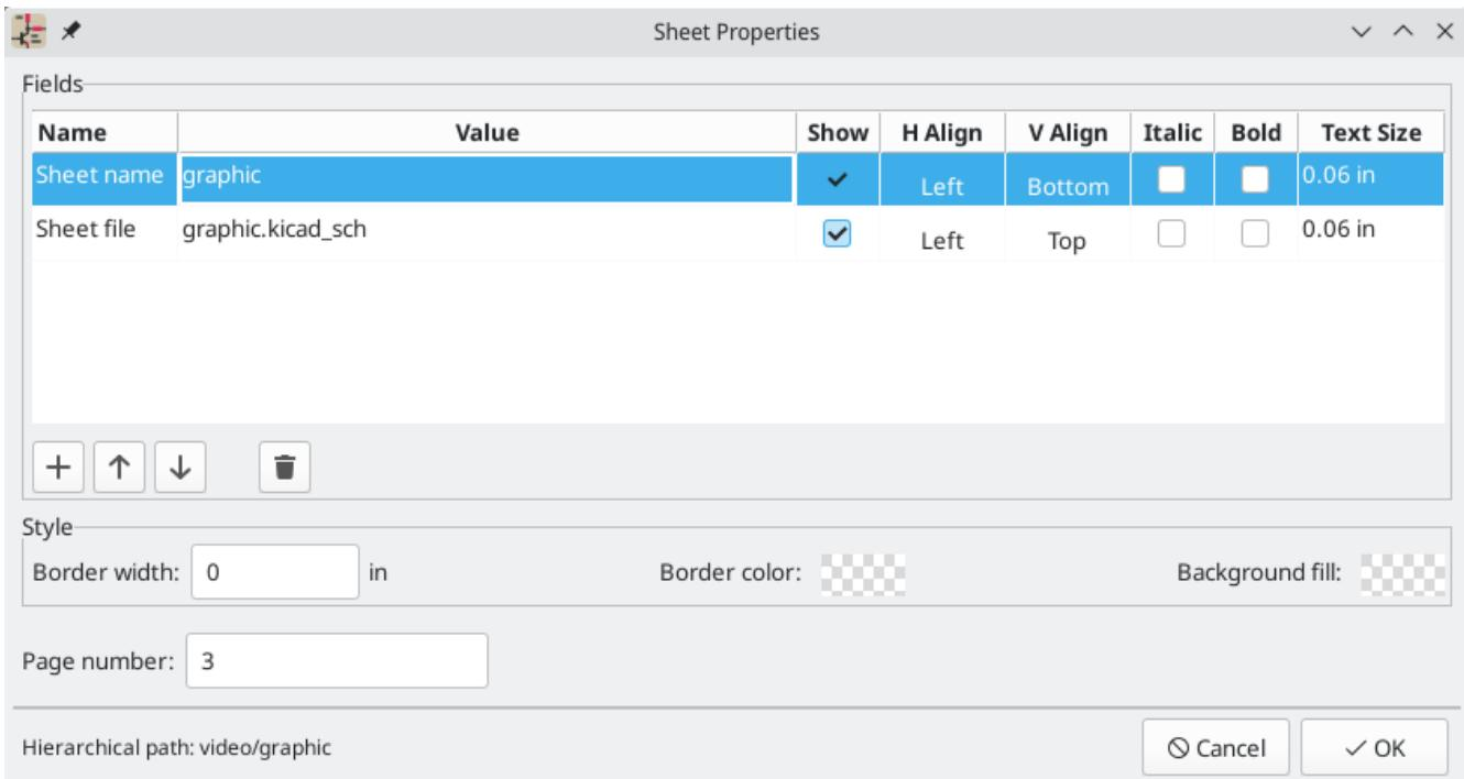
The **sheet name** must be unique, as it is used in the full net name for any nets in the subsheet. For example, a net with the local label `net1` in the sheet `sheet1` would have a full net name of `/sheet1/net1`. The sheet name is also used to refer to the sheet in various places in the GUI, including the [title block](#) and the [hierarchy navigator](#).
