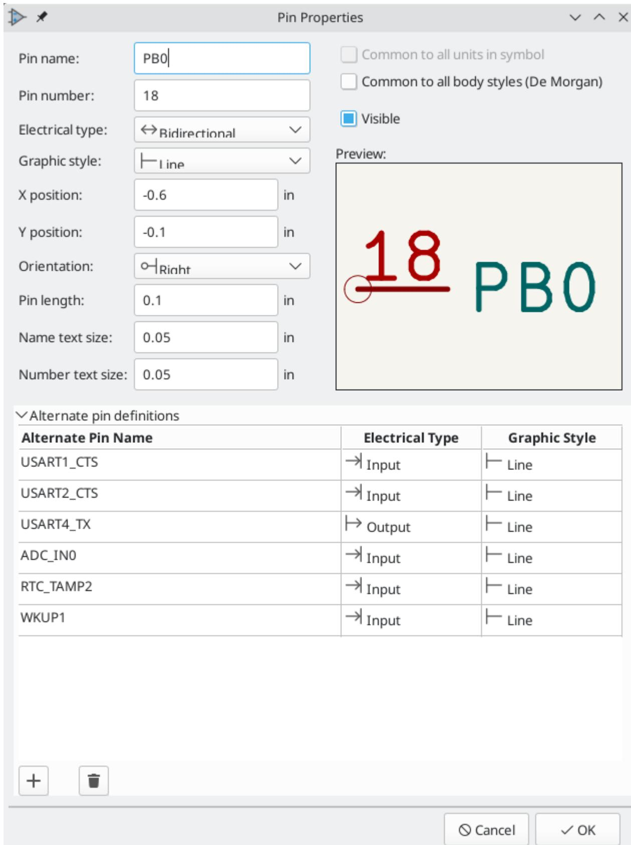
Alternate pin definitions are selected in the Schematic Editor once the symbol has been placed in the schematic. The alternate pin is assigned in the Alternate Pin Assignments tab of the Symbol Properties dialog. Alternate definitions are selectable in the dropdown in the Alternate Assignment column.
