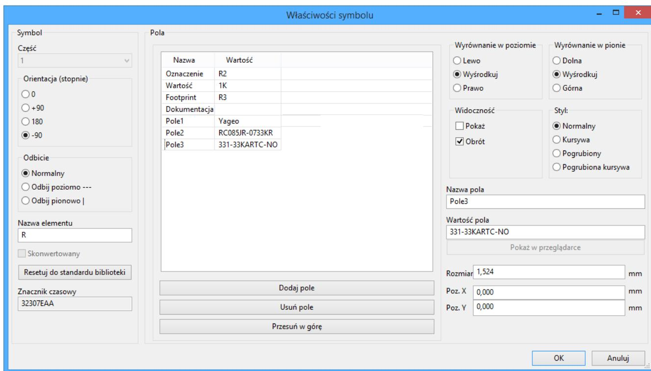
The Symbol Properties window displays all the fields of a symbol in a table. New fields can be added, and existing fields can be deleted, edited, reordered, moved, or resized.
