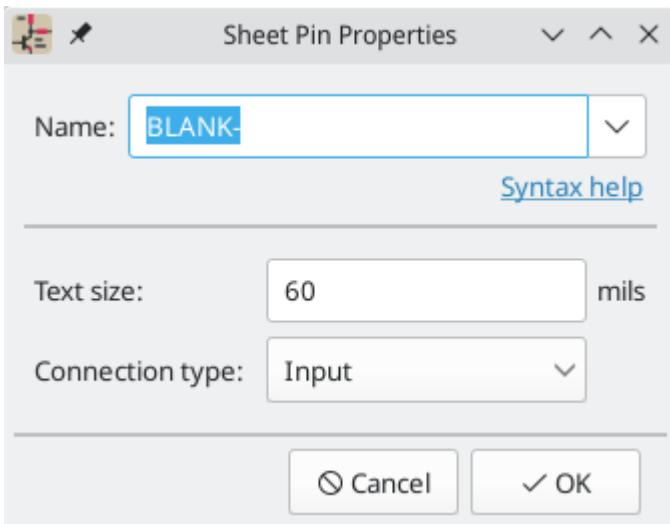
The sheet pin's **name** can be edited in the textbox or by selecting from the dropdown list of hierarchical labels in the subsheet. A sheet pin's name has to match the corresponding hierarchical label in the subsheet, so if a pin name is changed the label must change as well.
