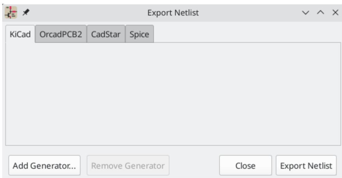
KiCad supports exporting netlists in several formats: KiCad, OrcadPCB2, CADSTAR, and Spice. Each format can be selected by selecting the corresponding tab at the top of the window. Some netlist formats have additional options.
