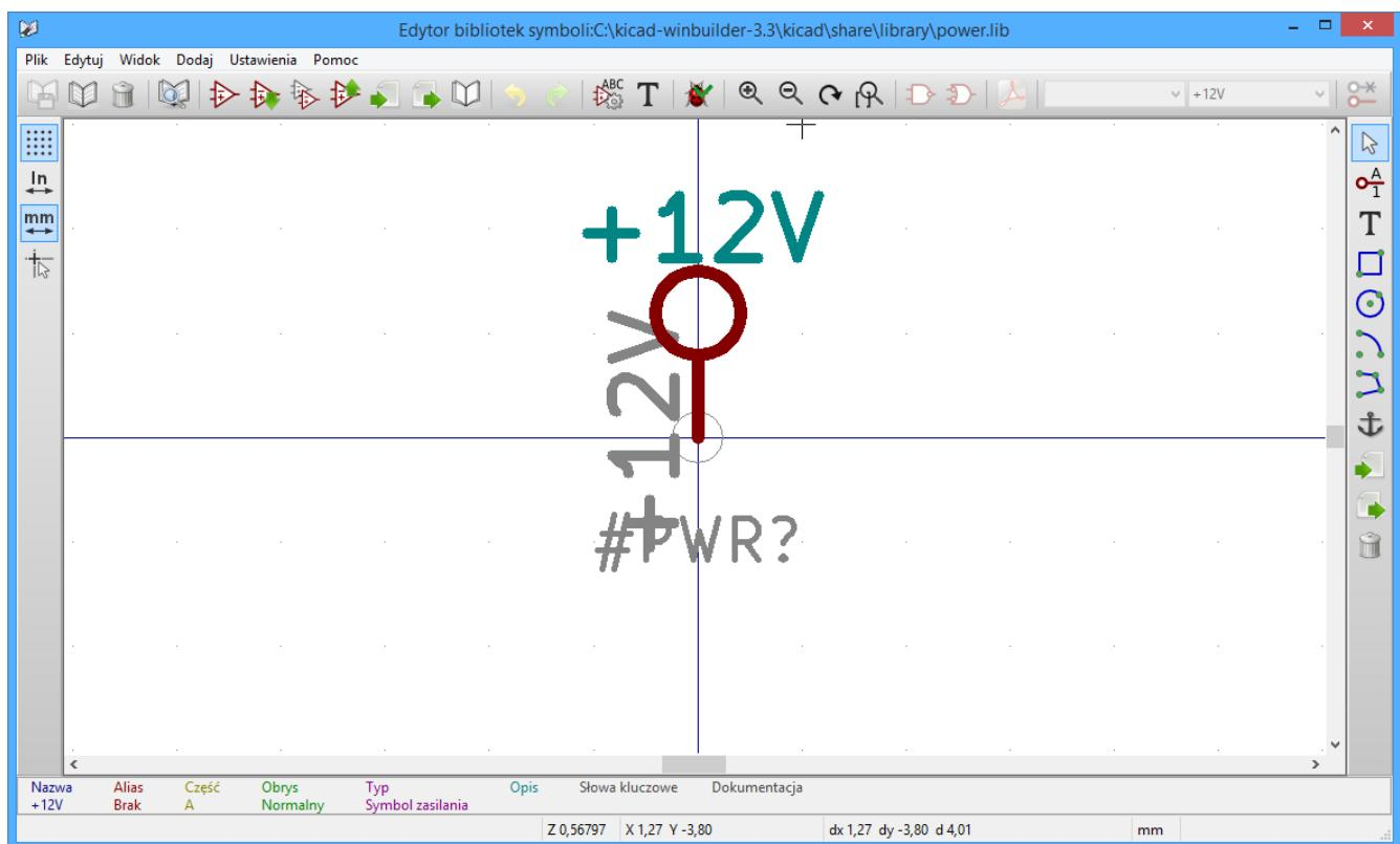
Power port symbols consist of a pin of type "Power input" that is marked invisible. They must also have the "Define as power symbol" property checked. [Invisible power input pins](#) have a special property of making implicit global connections based on the pin name.
