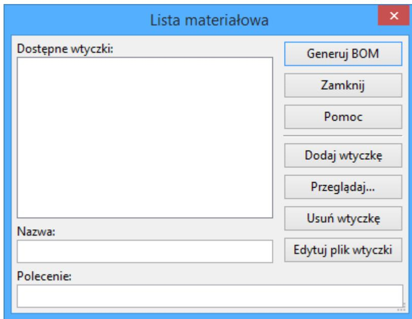
The BOM tool uses an external script to process the design information into the desired output format. Several BOM generator scripts are included with KiCad, and users can also create their own. BOM generator scripts generally use Python or XSLT, but other tools can be used as long as you can specify a [command line](#) for KiCad to execute when running the generator.
