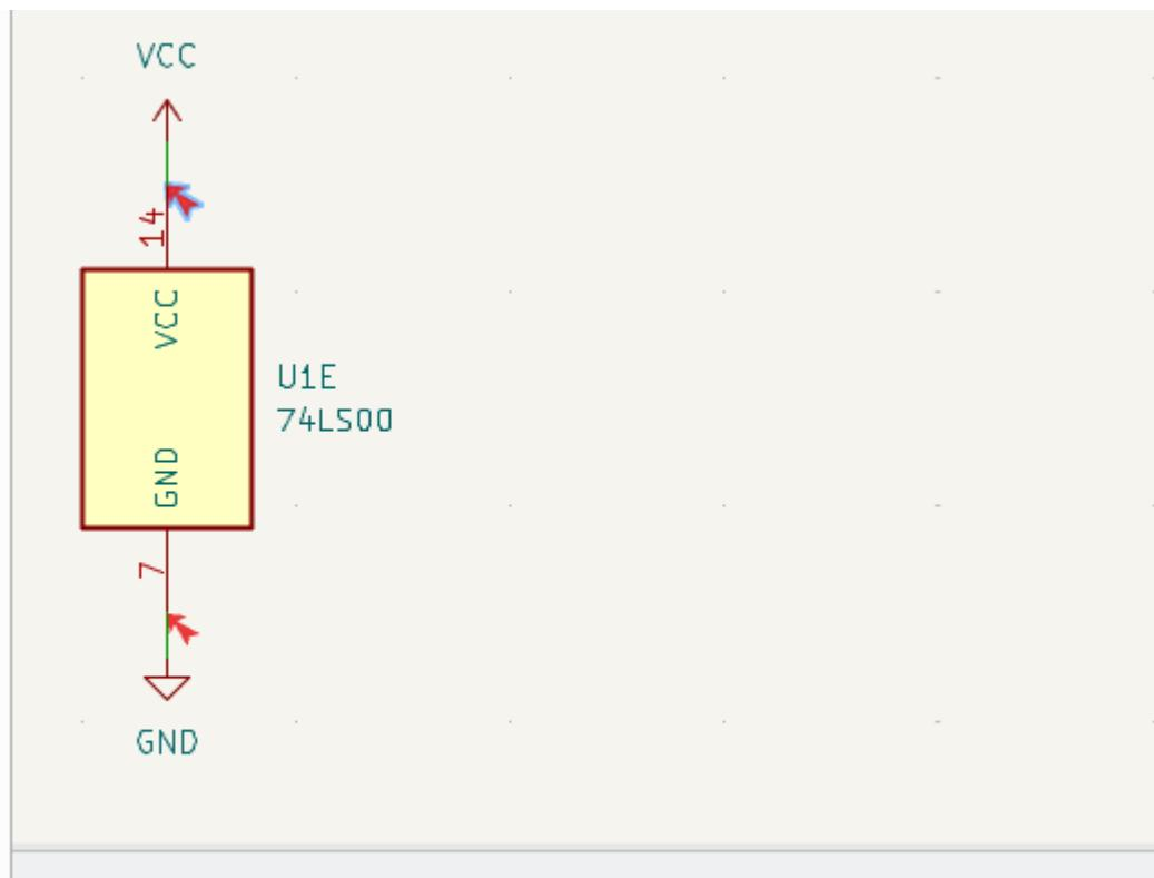
To avoid this warning, connect the net to `PWR_FLAG` symbol on such a power net as shown in the following example. The `PWR_FLAG` symbol is found in the `power` symbol library. Alternatively, connect any power output pin to the net; `PWR_FLAG` is simply a symbol with a single power output pin.
