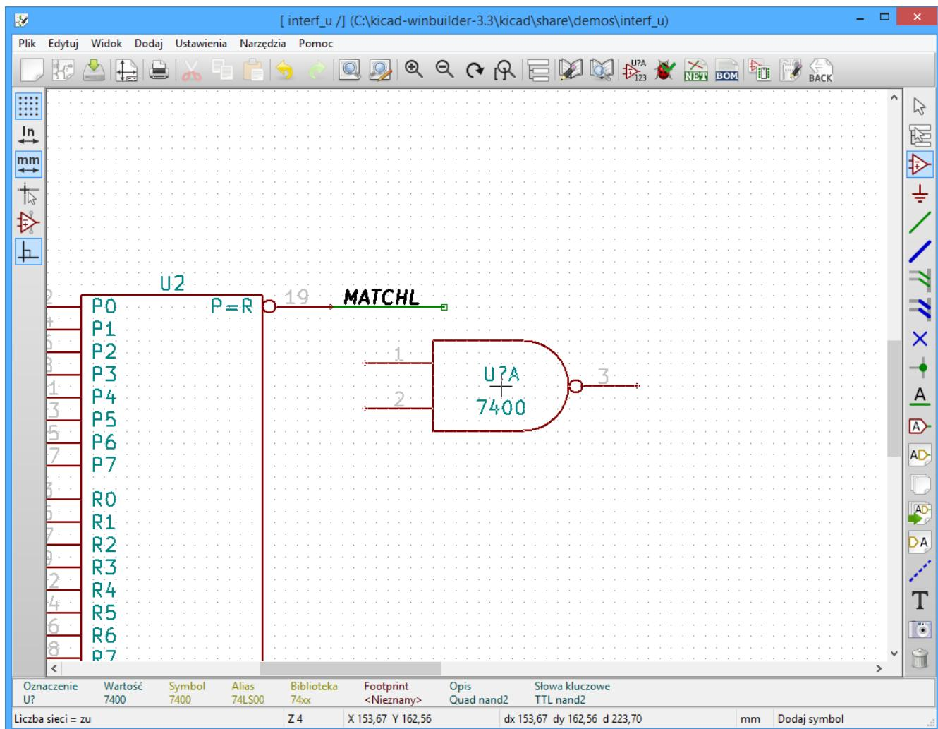
If the **Place repeated copies** option is checked, after placing a symbol KiCad will start placing another copy of the symbol. This process continues until the user presses **Esc**.
