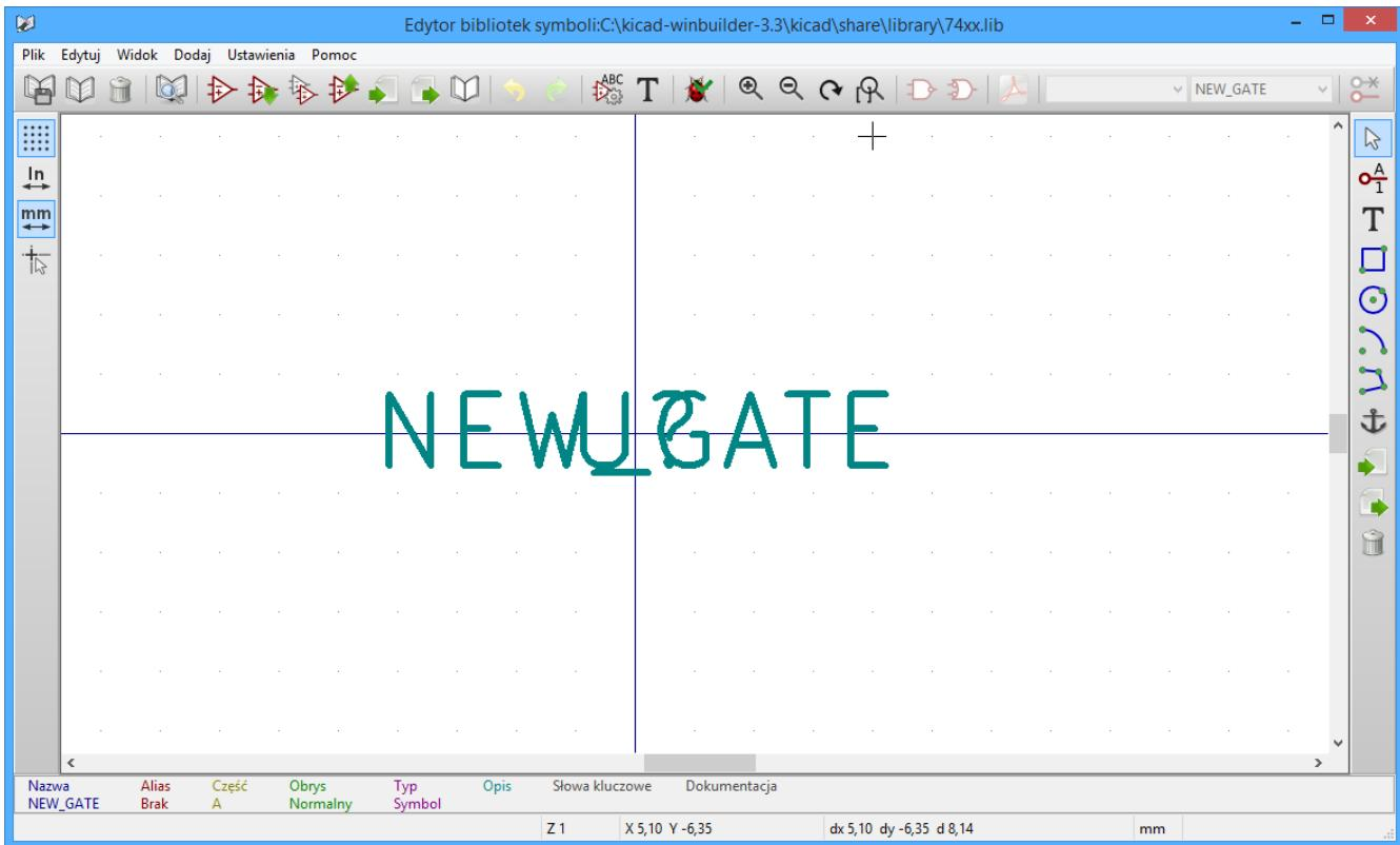
The blue cross in the center is the symbol anchor, which specifies the symbol origin i.e. the coordinates (0, 0). The anchor can be repositioned by selecting the icon and clicking on the new desired anchor position.
