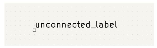
The connection point's position relative to the label text can be changed by choosing a different label orientation in the label's properties, or by mirroring/rotating the label.
