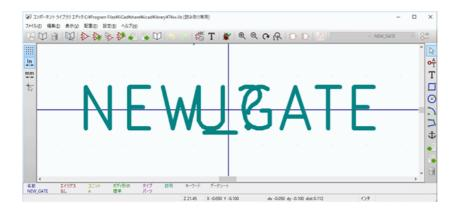
The blue cross in the center is the symbol anchor, which specifies the symbol origin i.e. the coordinates (0, 0). The anchor can be repositioned by selecting the \*@@ icon and clicking on the new desired anchor position.
