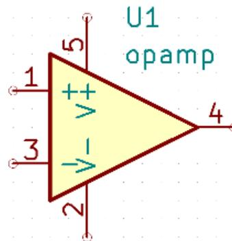
To match the symbol pins to the Spice model nodes shown above, one needs to use an alternate node sequence option with value: "1 3 5 2 4". It is a list of pin numbers corresponding to the Spice model nodes order.
