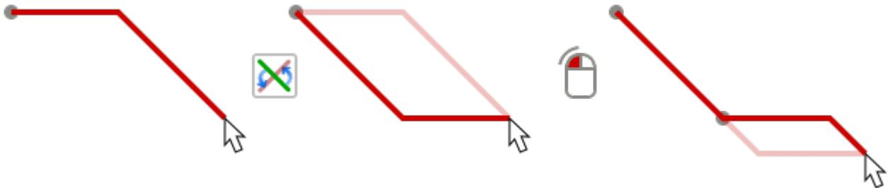
Holding *Ctrl* while routing in the non-legacy canvases constrains the routing to a single horizontal or vertical segment. Switching posture changes to a single diagonal segment. Holding *Shift* while routing removes the *snap to object* gravity.
