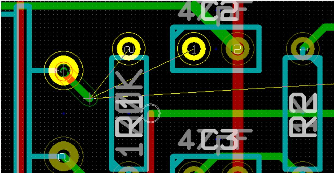
As you move the mouse, a track is drawn connecting the origin of the track with the current mouse position. The track will be drawn with at most two segments (for example, rightwards, then a switch to diagonally). Clicking while routing locks in the corner node.
