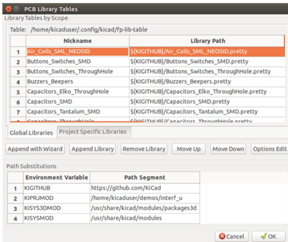
In order to use a footprint library, it must first be added to either the global table or the project specific table. The project specific table is only applicable when a board file is open.
