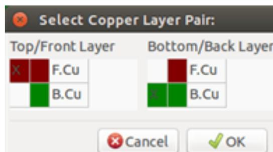
When a via is placed the working (active) layer is automatically switched to the alternate layer of the layer pair used for the vias (unless *Shift* is held when adding the via).
