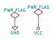
This will avoid the classic schematic checking warning: Pin connected to some other pins but no pin to drive it.
