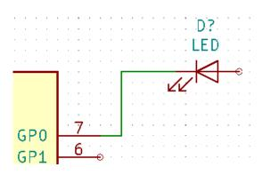
33. Repeat this process and wire up all the other components as shown below. To terminate a wire just double-click. When wiring up the VCC and GND symbols, the wire should touch the bottom of the VCC symbol and the middle top of the GND symbol. See the screenshot below.
